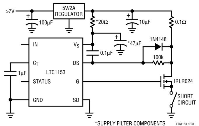
Figure 8. Supply Filter for Current Limited Supplies
