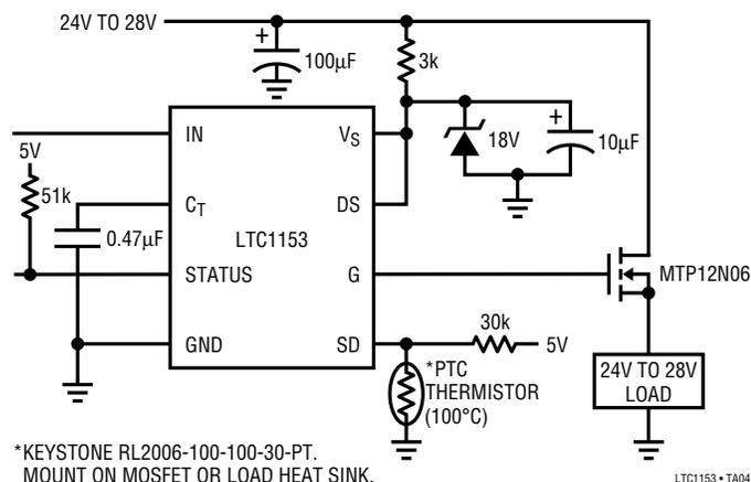
**24V to 28V Over-Temperature Circuit Breaker with Bootstrapped Supply**
