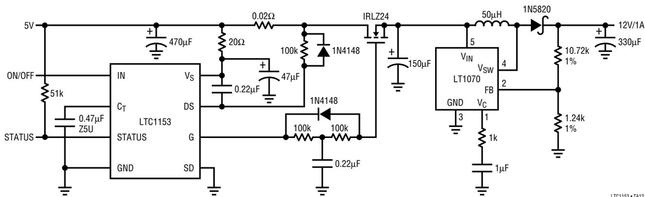
**12V Step-Up Regulator with 1A Circuit Breaker (Post Regulator), Breaker Status Feedback and Ramped Output**
