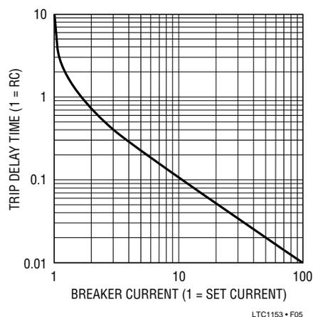
Figure 5. Trip Delay Time vs Breaker Current
