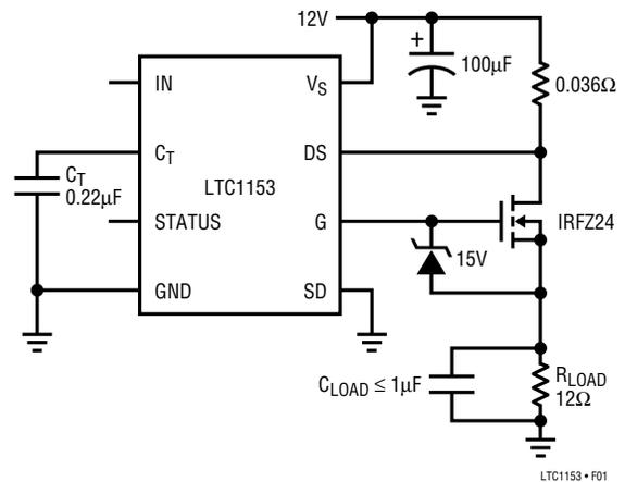
Figure 1. Protecting Resistive Loads
