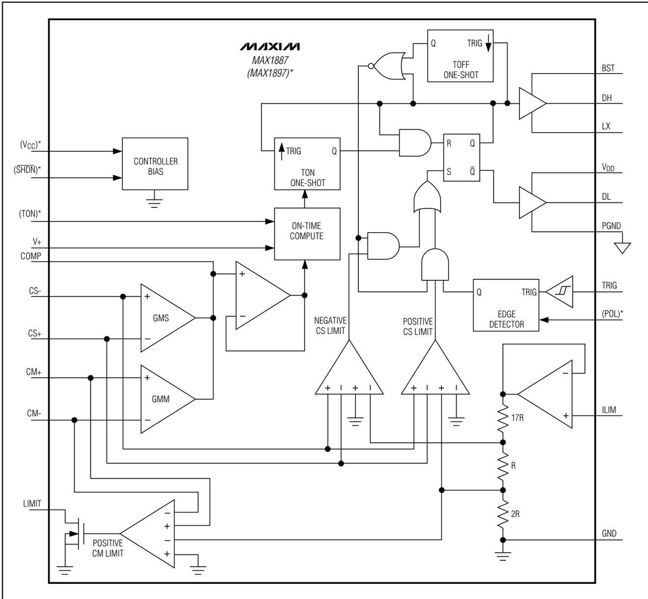
Figure 2. Functional Diagram
