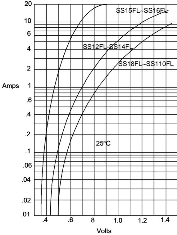
Instantaneous Forward Current - Amperes *versus*
