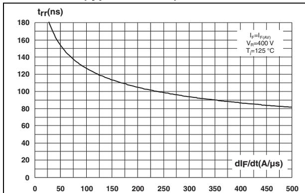
Figure 6. Reverse recovery charges versus di\_F/dt (typical values)
