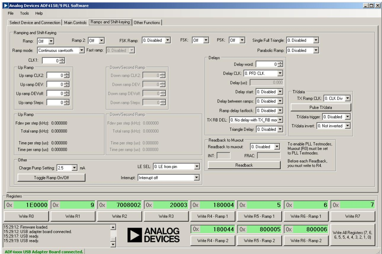
Figure 9. Software—Ramp Controls
