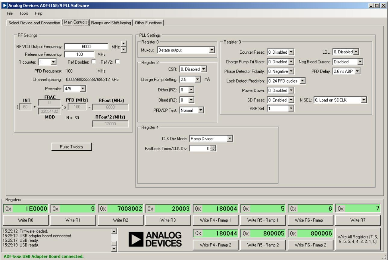
Figure 7. Software—Main Controls
