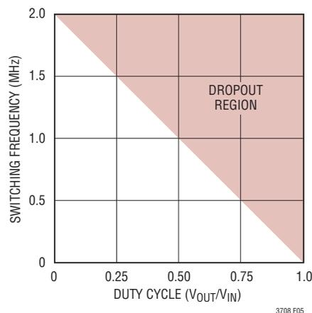
Figure 5. Maximum Switching Frequency vs Duty Cycle
