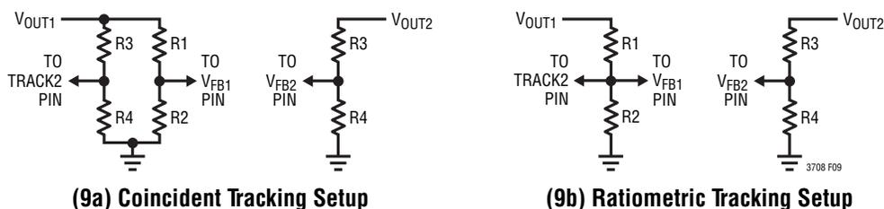
Figure 9. Setup for Coincident and Ratiometric Tracking
