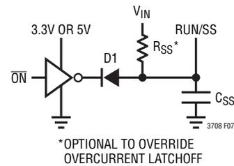
Figure 7. RUN/SS Pin Interfacing with Latchoff Defeated
