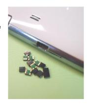
An advanced feature of the PolyZen devices is that the Zener diode is thermally coupled to a resistively non-linear, polymer PTC (positive temperature coefficient) substrate. The PTC substrate is fully integrated into the device, and is electrically in series between  $V_{\text{IN}}$  and the diode clamped  $V_{\text{OUT}}$ .
