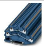
Double-level terminal block, Cross section: 0.14 mm² - 1.5 mm², AWG: 26 - 14, Connection type: Push-in connection, Width: 3.5 mm, Color: blue, Mounting type: NS 35/7,5, NS 35/15
