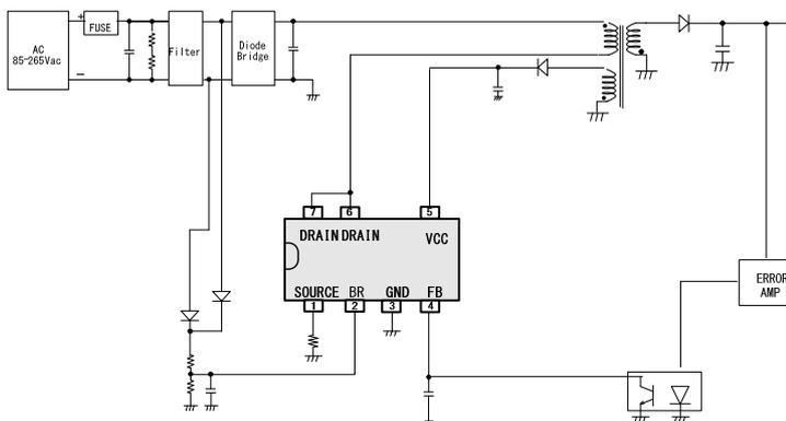
Figure 1. Application circuit
