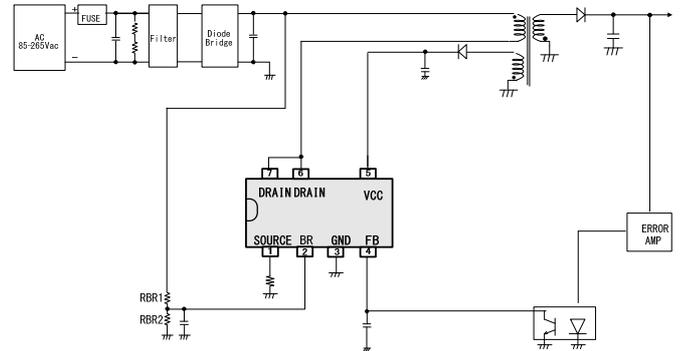
Figure 16(b). DC voltage monitor setting
