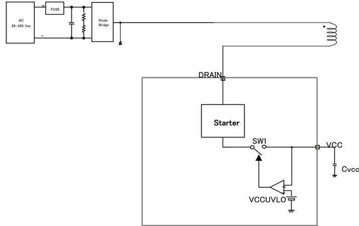
Figure 4. Block diagram of start circuit
