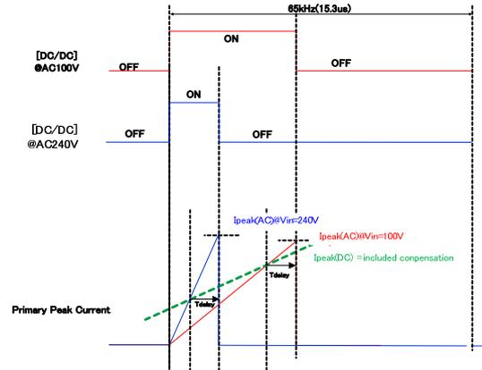
Figure13. built-in AC compensation voltage
