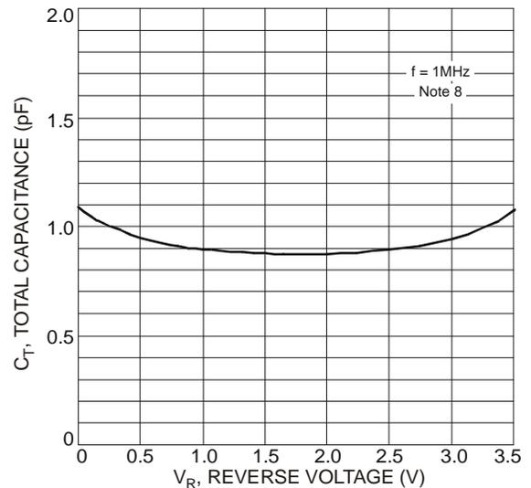
Figure 6 Typical Total Capacitance vs. Reverse Voltage
