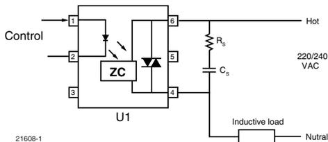
Fig. 11 - Basic Direct Load Driving Circuit
