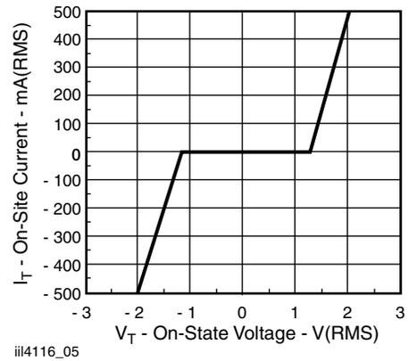
Fig. 5 - On-State Terminal Voltage vs. Terminal Current
