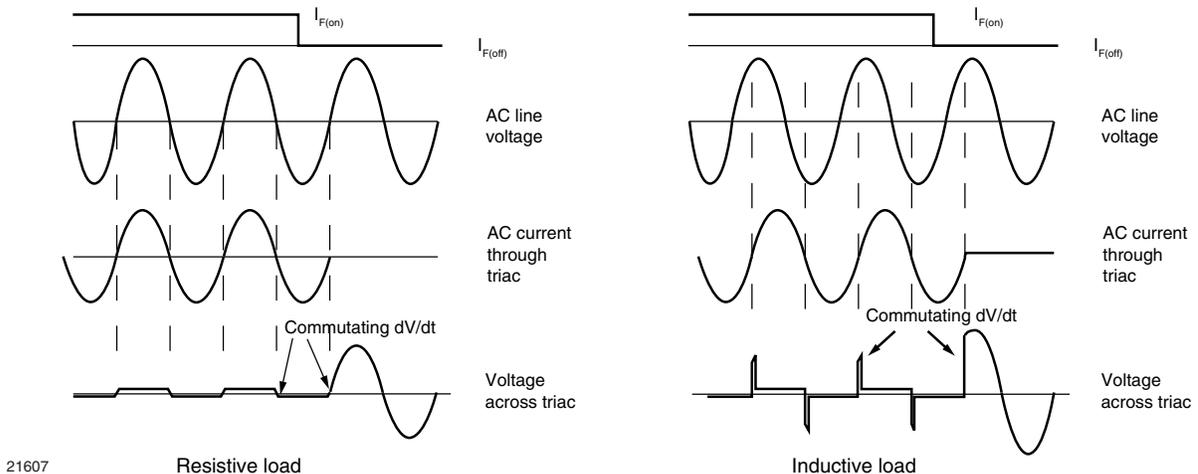
Fig. 8 - Waveforms of Resistive and Inductive Loads
