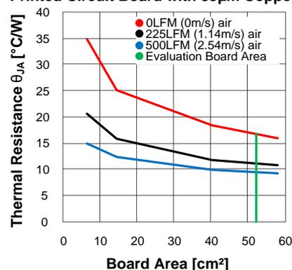
For  $\theta_{JA} < 17.1^{\circ}C/W$  and only natural convection (i.e. no air flow), the minimum PCB area can be smaller than 9cm<sup>2</sup>. This corresponds to a square board with 3cm x 3cm copper area, 4 layers, and 35 $\mu$ m copper thickness. Higher copper thickness will further improve the overall thermal performance. Note that thermal vias should be placed under the IC package to easily transfer heat from the top layer of the PCB to the inner layers and the bottom layer.
