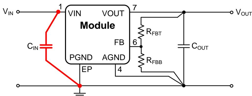
Based on those considerations, the path of the input capacitor  $C_{IN}$  is the most critical one to generate high frequency noise on  $V_{in}$ . Therefore place  $C_{IN}$  as close as possible to the MagI<sup>3</sup>C power module  $V_{IN}$  and PGND exposed pad EP. This will minimize the high  $di/dt$  area and reduce radiated EMI. Additionally, grounding for both the input and output capacitor should consist of a localized top side plane that connects to the PGND exposed pad.
