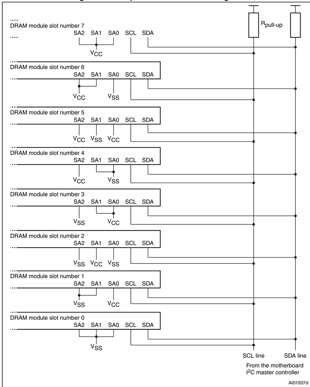
1. SA0, SA1 and SA2 are wired at each DRAM module slot in a binary sequence for a maximum of 8 devices.
