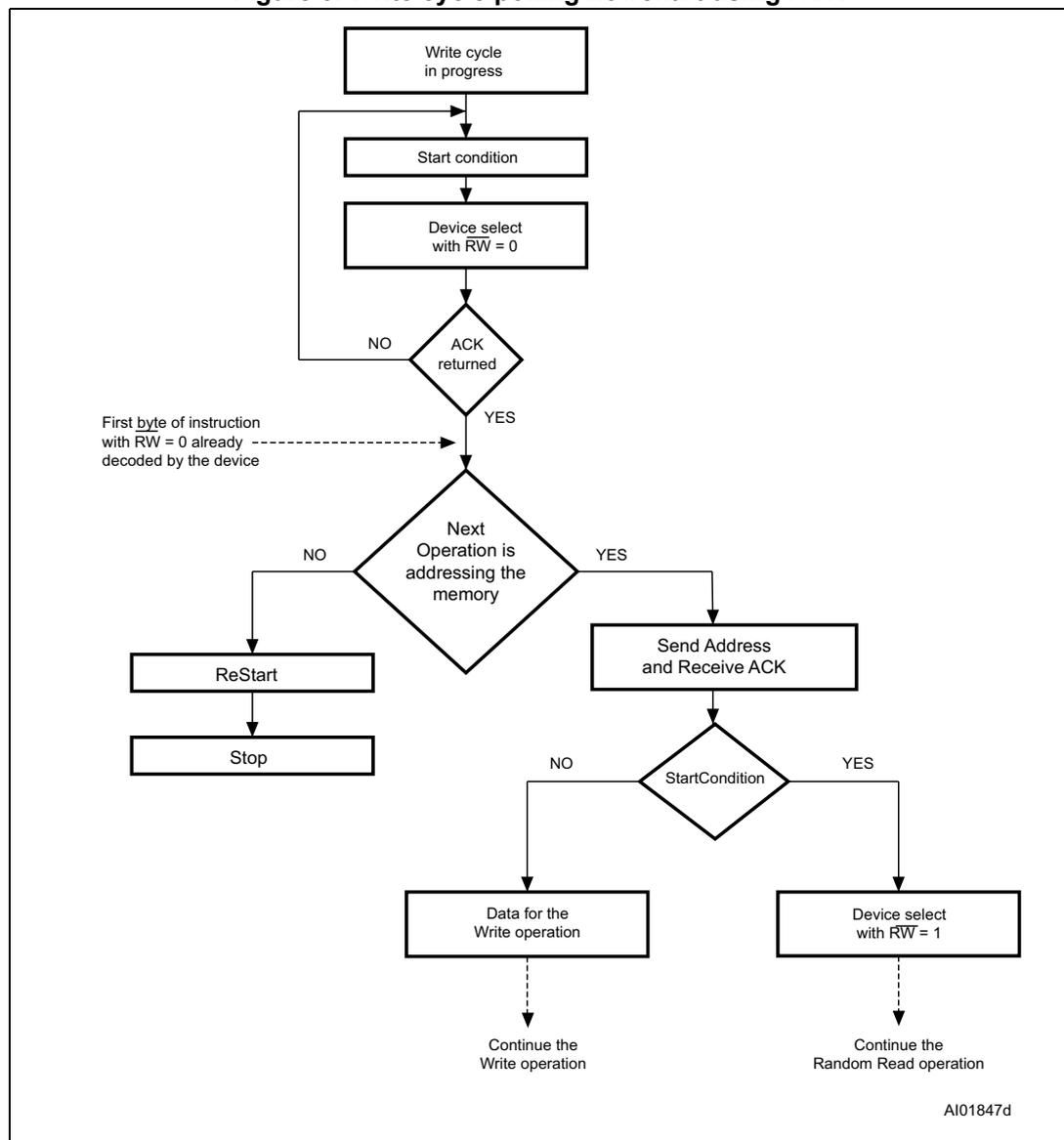
During the internal Write cycle, the device disconnects itself from the bus, and writes a copy of the data from its internal latches to the memory cells. The maximum Write time ( $t_w$ ) is shown in [Table 13](#), but the typical time is shorter. To make use of this, a polling sequence can be used by the bus master.
