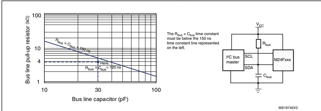
**Figure 13. Maximum  $R_{bus}$  value versus bus parasitic capacitance ( $C_{bus}$ ) for an I<sup>2</sup>C bus at maximum frequency  $f_c = 400$  kHz**
