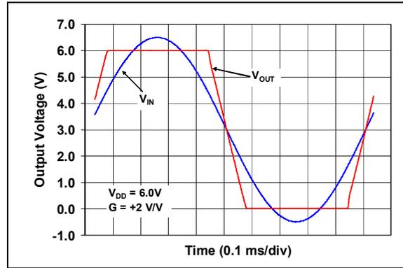
**FIGURE 2-34:** The MCP6051/2/4 Shows No Phase Reversal.
