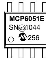
8-Lead 2x3 TDFN (MCP6051, MCP6052)
