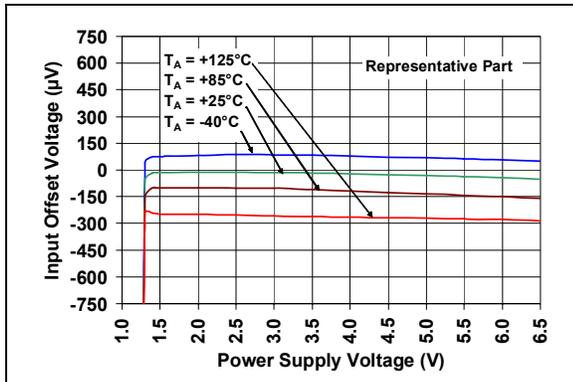
**FIGURE 2-8:** Input Offset Voltage vs. Power Supply Voltage.
