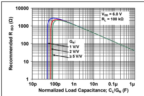
**FIGURE 4-5:** Recommended  $R_{ISO}$  Values for Capacitive Loads.
