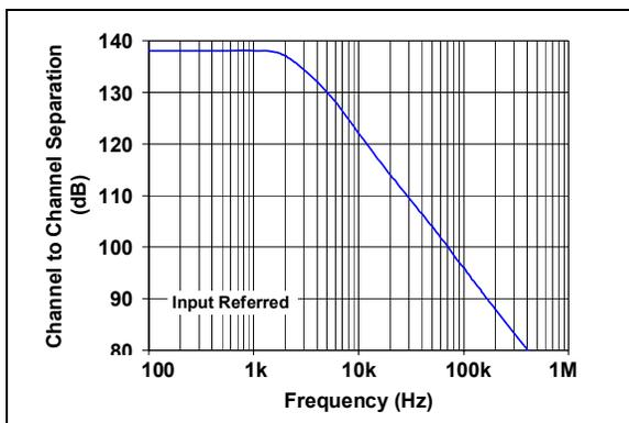
**FIGURE 2-21:** Channel-to-Channel Separation vs. Frequency (MCP6052/4 only).
