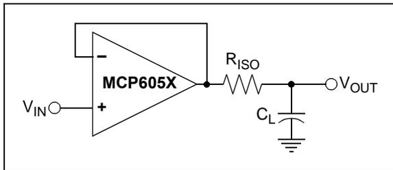
**FIGURE 4-4:** Output Resistor,  $R_{ISO}$  Stabilizes Large Capacitive Loads.
