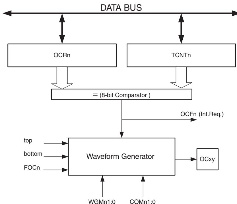
The OCR0 Register is double buffered when using any of the Pulse Width Modulation (PWM) modes. For the normal and Clear Timer on Compare (CTC) modes of operation, the double buffering is disabled. The double buffering synchronizes the update of the OCR0 Compare Register to either top or bottom of the counting sequence. The synchronization prevents the occurrence of odd-length, non-symmetrical PWM pulses, thereby making the output glitch-free.
