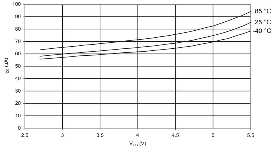
**Figure 209.** Programming Current vs.  $V_{CC}$
