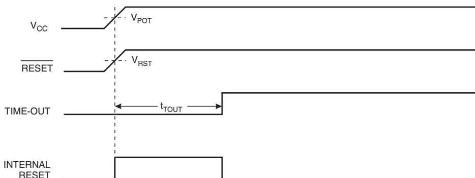
**Figure 24.** MCU Start-up,  $\overline{RESET}$  Extended Externally
