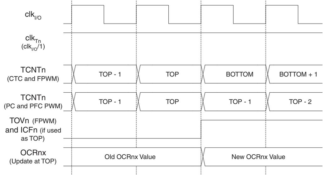
Figure 58 shows the same timing data, but with the prescaler enabled.
