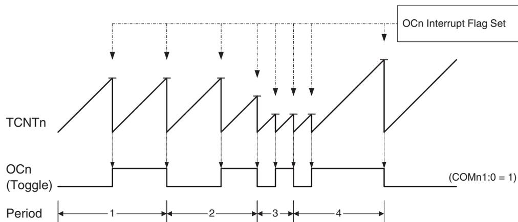
An interrupt can be generated each time the counter value reaches the TOP value by using the OCF0 flag. If the interrupt is enabled, the interrupt handler routine can be used for updating the TOP value. However, changing the TOP to a value close to BOTTOM when the counter is running with none or a low prescaler value must be done with care since the CTC mode does not have the double buffering feature. If the new value written to OCR0 is lower than the current
