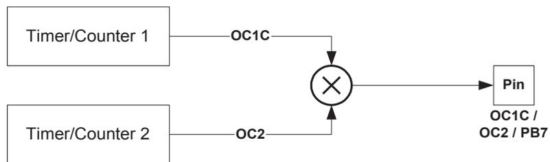
When the modulator is enabled, the two output compare channels are modulated together as shown in the block diagram (Figure 72).
