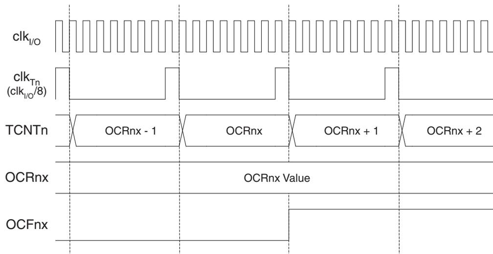
Figure 57 shows the count sequence close to TOP in various modes. When using phase and frequency correct PWM mode the OCRnx Register is updated at BOTTOM. The timing diagrams will be the same, but TOP should be replaced by BOTTOM, TOP-1 by BOTTOM+1 and so on. The same renaming applies for modes that set the TOVn flag at BOTTOM.
