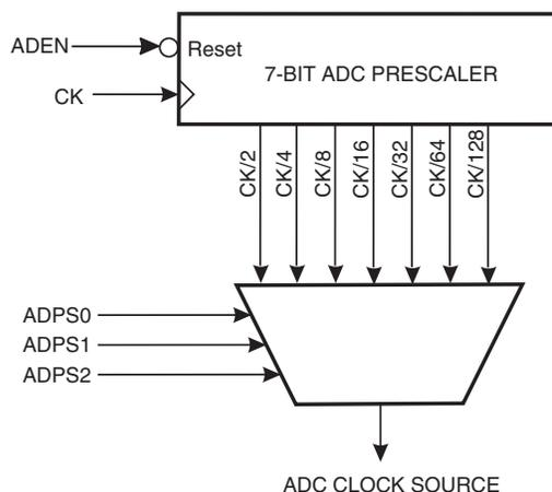
By default, the successive approximation circuitry requires an input clock frequency between 50kHz and 200kHz to get maximum resolution. If a lower resolution than 10 bits is needed, the input clock frequency to the ADC can be higher than 200kHz to get a higher sample rate.
