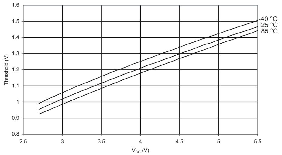
**Figure 188.** I/O Pin Input Hysteresis vs.  $V_{CC}$
