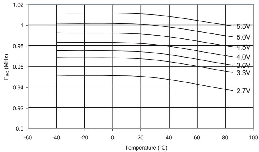
**Figure 194.** Calibrated 1MHz RC Oscillator Frequency vs.  $V_{CC}$
