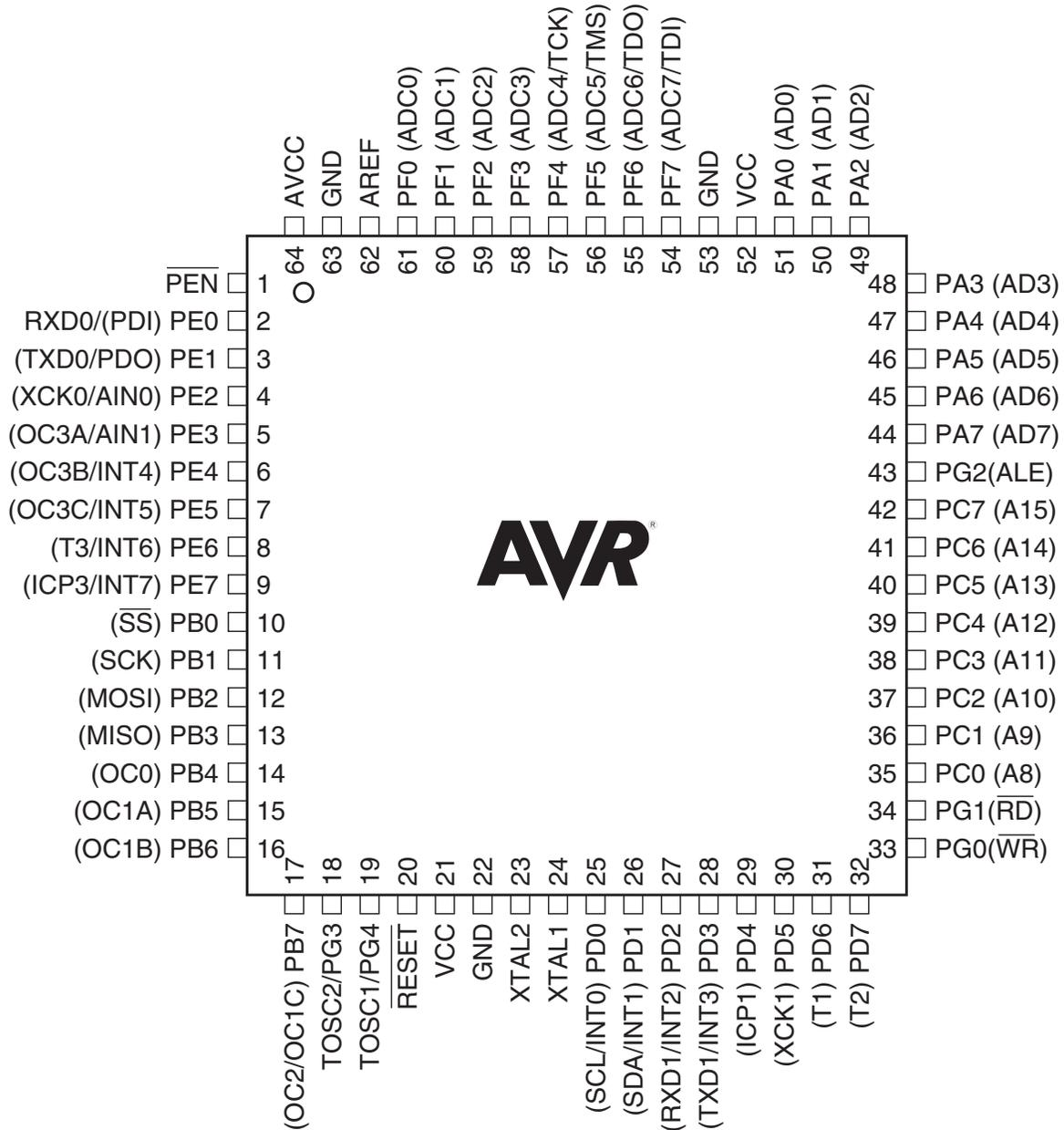
Note: The Pinout figure applies to both TQFP and MLF packages. The bottom pad under the QFN/MLF package should be soldered to ground.
