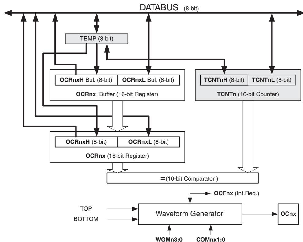
The OCRnx Register is double buffered when using any of the twelve *Pulse Width Modulation* (PWM) modes. For the normal and *Clear Timer on Compare* (CTC) modes of operation, the double buffering is disabled. The double buffering synchronizes the update of the OCRnx Compare Register to either TOP or BOTTOM of the counting sequence. The synchronization prevents the occurrence of odd-length, non-symmetrical PWM pulses, thereby making the output glitch-free.
