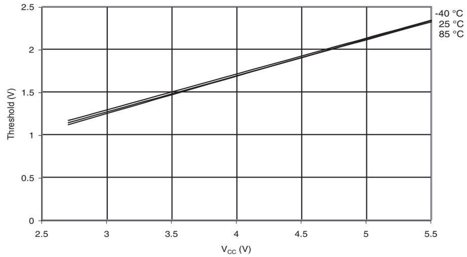
**Figure 216.** Reset Input Pin Hysteresis vs.  $V_{CC}$
