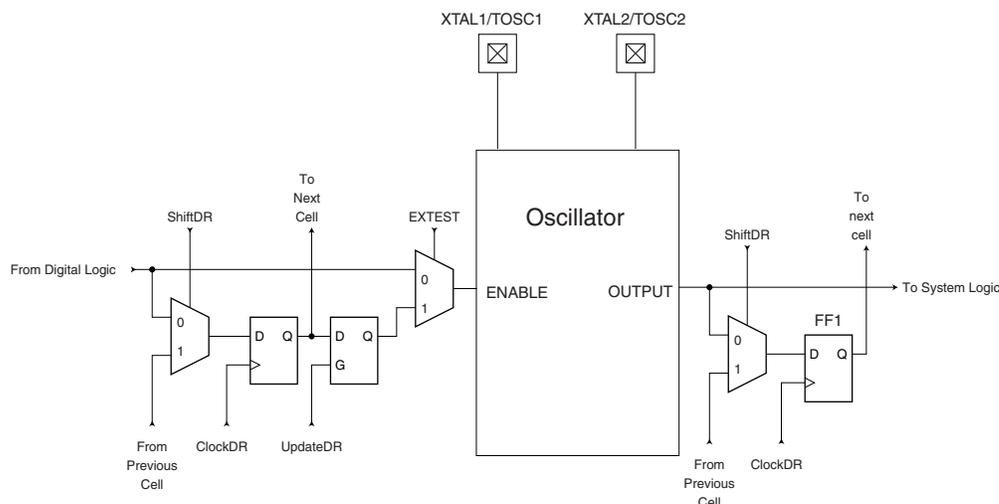
Table 102 summarizes the scan registers for the external clock pin XTAL1, oscillators with XTAL1/XTAL2 connections as well as 32kHz Timer Oscillator.
