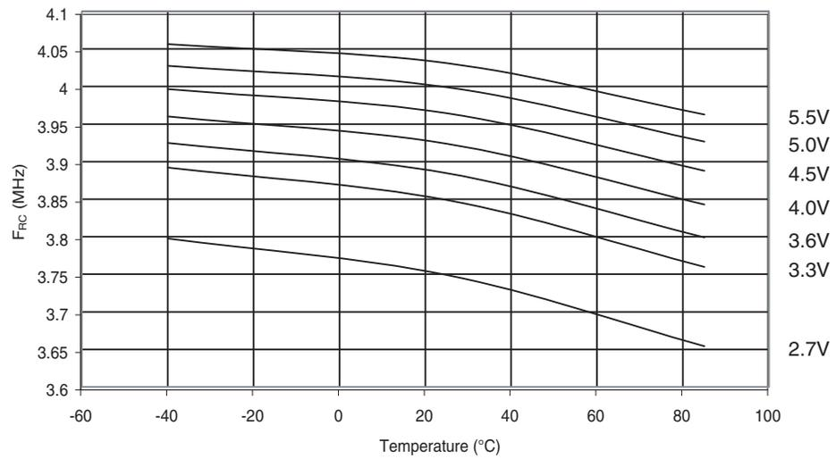
**Figure 200.** Calibrated 4MHz RC Oscillator Frequency vs.  $V_{CC}$
