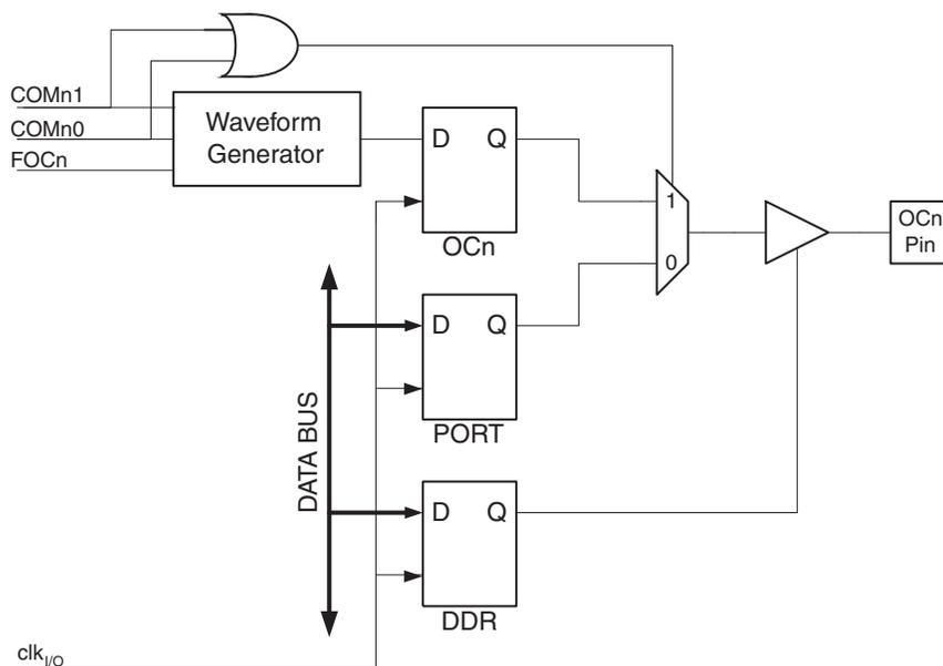
The general I/O port function is overridden by the output compare (OC2) from the waveform generator if either of the COM21:0 bits are set. However, the OC2 pin direction (input or output) is still controlled by the Data Direction Register (DDR) for the port pin. The Data Direction Register bit for the OC2 pin (DDR\_OC2) must be set as output before the OC2 value is visible on the pin. The port override function is independent of the Waveform Generation mode.
