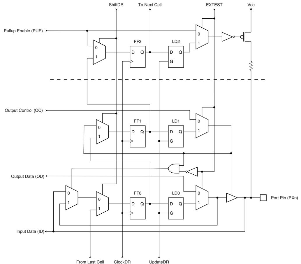
**Figure 126.** Additional Scan Signal for the Two-wire Interface
