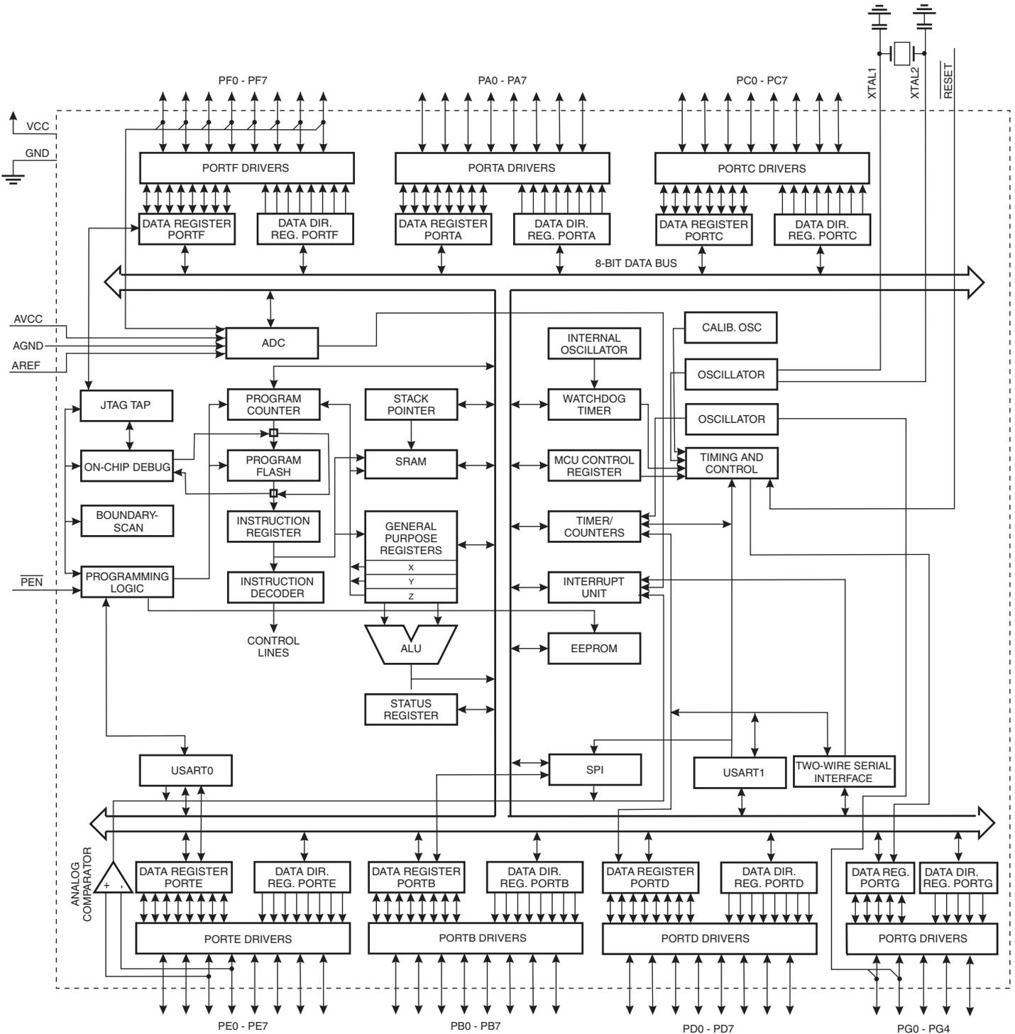
The Atmel® AVR® core combines a rich instruction set with 32 general purpose working registers. All the 32 registers are directly connected to the Arithmetic Logic Unit (ALU), allowing two independent registers to be accessed in one single instruction executed in one clock cycle. The resulting architecture is more code efficient while achieving throughputs up to ten times faster than conventional CISC microcontrollers.
