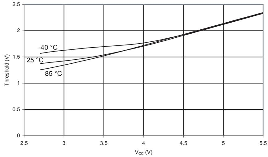
**Figure 215.** Reset Input Threshold Voltage vs.  $V_{CC}$  (VIL, Reset Pin Read as '0')
