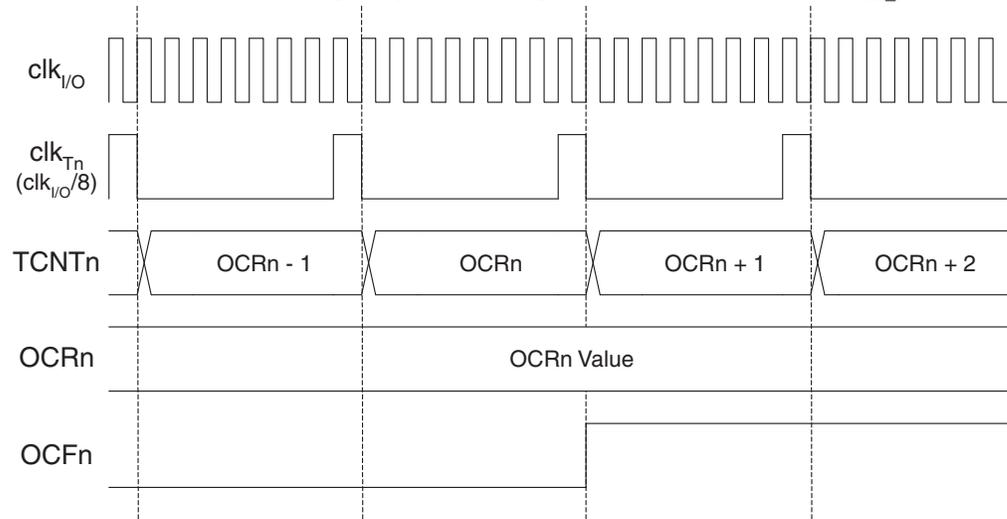
Figure 71 shows the setting of OCF2 and the clearing of TCNT2 in CTC mode.
