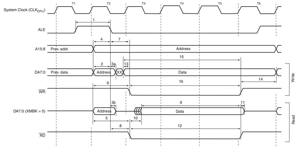
**Figure 160. External Memory Timing (SRWn1 = 1, SRWn0 = 1)<sup>(1)</sup>**
