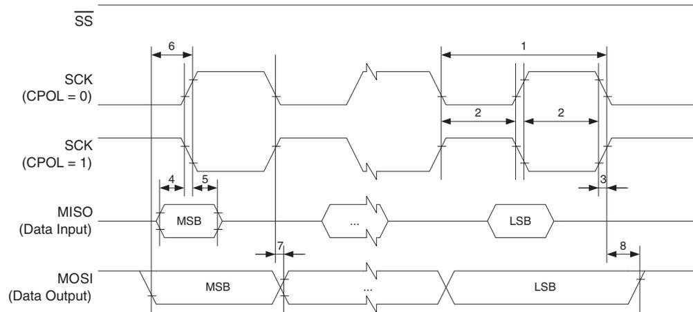
**Figure 156. SPI Interface Timing Requirements (Slave Mode)**
