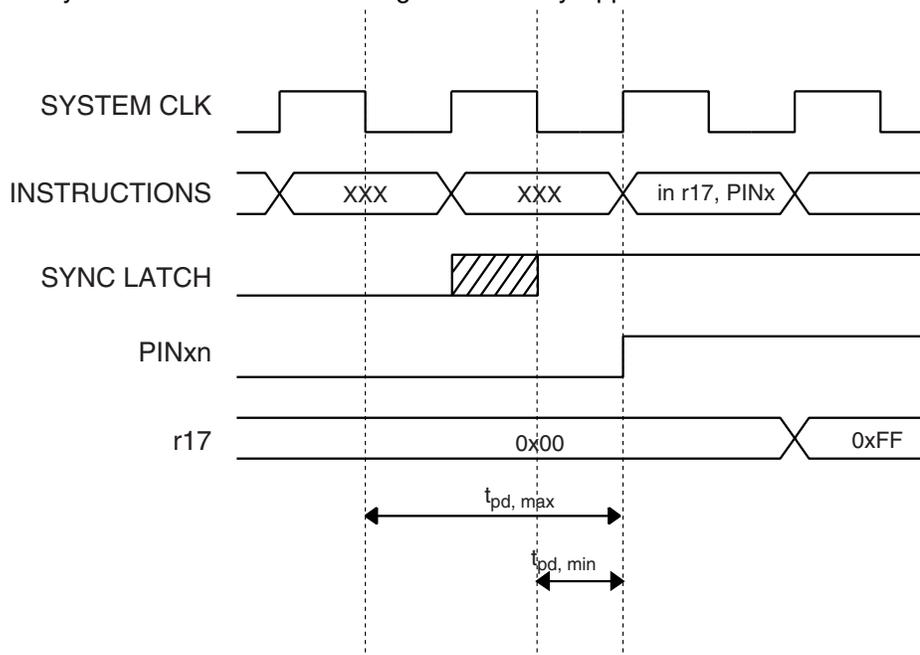
Consider the clock period starting shortly *after* the first falling edge of the system clock. The latch is closed when the clock is low, and goes transparent when the clock is high, as indicated by the
