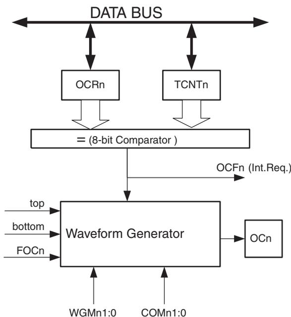
The OCR2 Register is double buffered when using any of the pulse width modulation (PWM) modes. For the normal and Clear Timer on Compare (CTC) modes of operation, the double buff-
