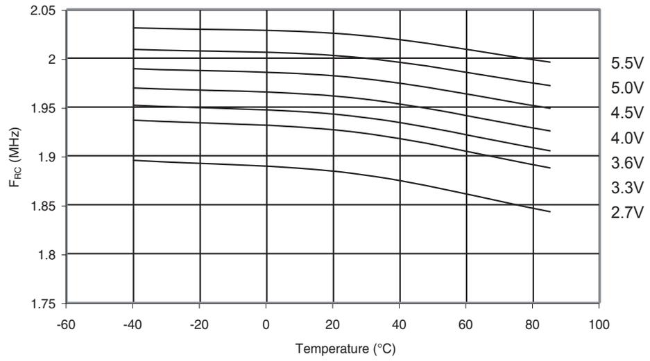
**Figure 197.** Calibrated 2MHz RC Oscillator Frequency vs. V<sub>CC</sub>
