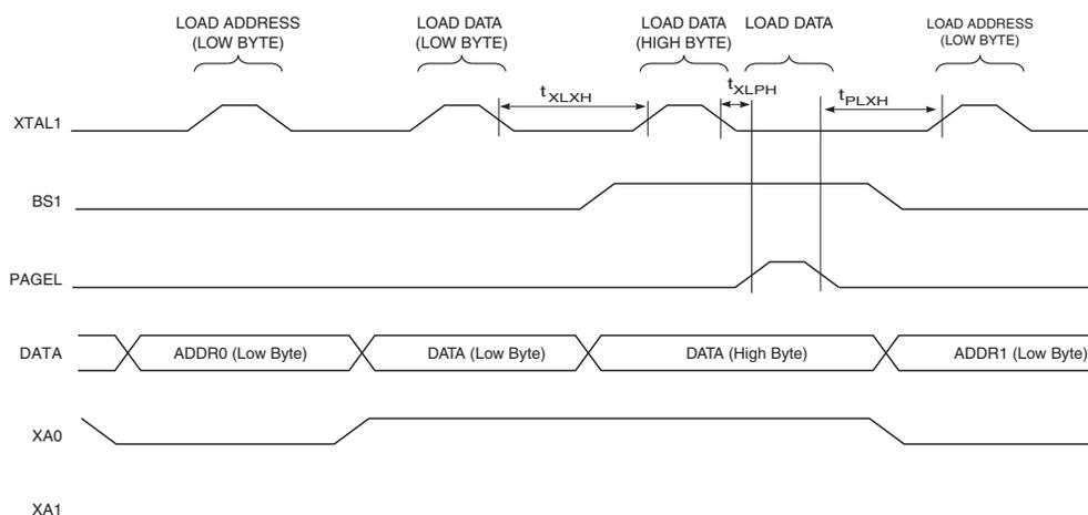
Note: The timing requirements shown in Figure 141 (i.e.  $t_{DVXH}$ ,  $t_{XHXL}$ , and  $t_{XLDX}$ ) also apply to loading operation.
