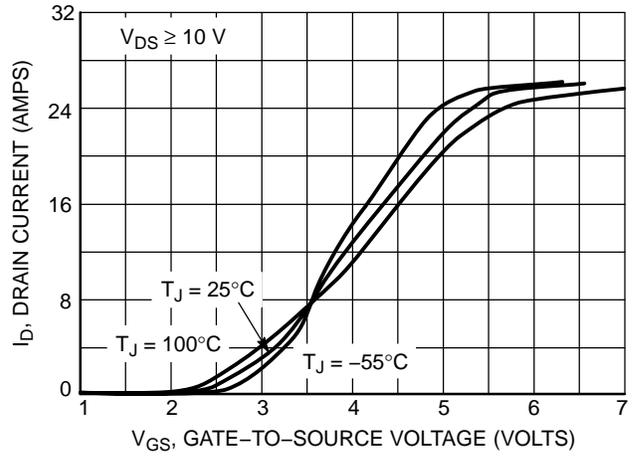
Figure 2. Transfer Characteristics
