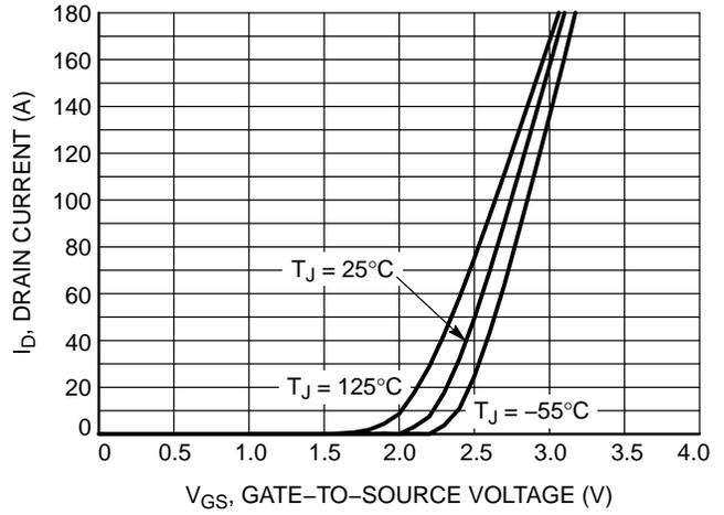
Figure 2. Transfer Characteristics
