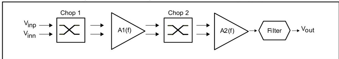
*Figure 38: "Block diagram in the time domain (step 1)"* shows step 1, the first clock cycle, where  $V_{io}$  is amplified in the normal way.
