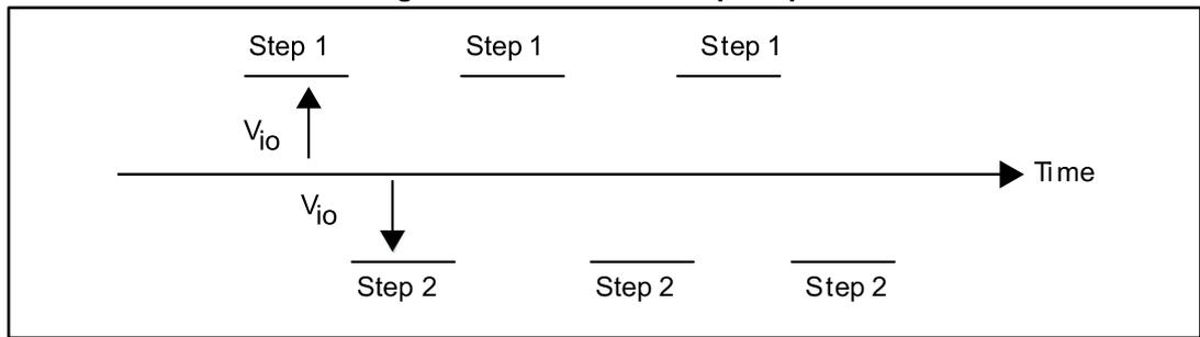
The low pass filter averages the output value resulting in the cancellation of the  $V_{io}$  offset.
