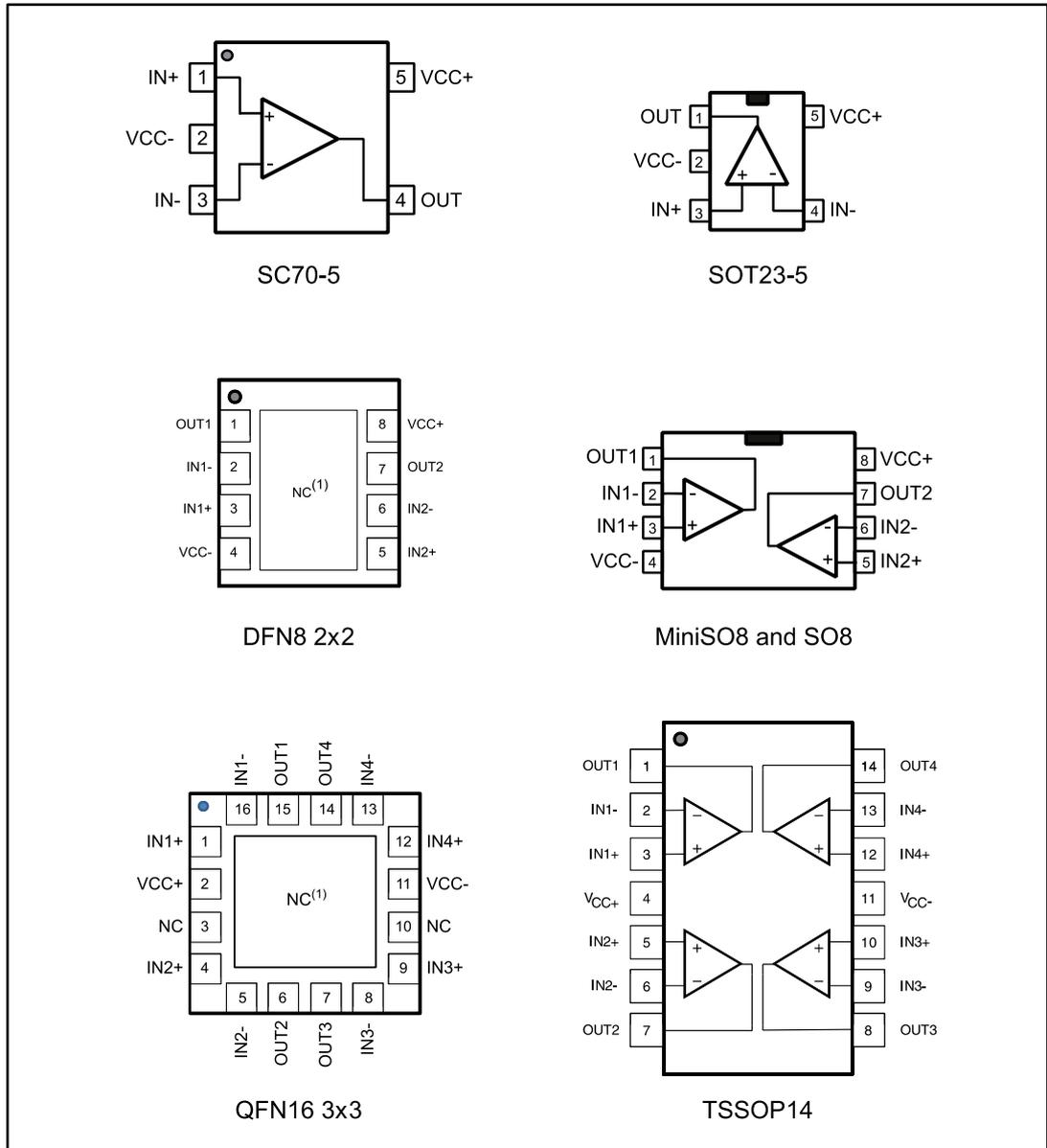
1. The exposed pads of the DFN8 2x2 and the QFN16 3x3 can be connected to VCC- or left floating.
