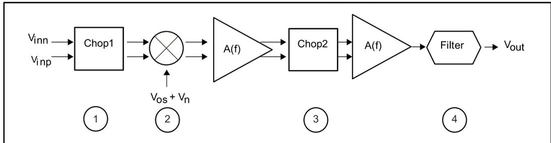
The modulation technique transposes the signal to a higher frequency where there is no  $1/f$  noise, and demodulate it back after amplification.
