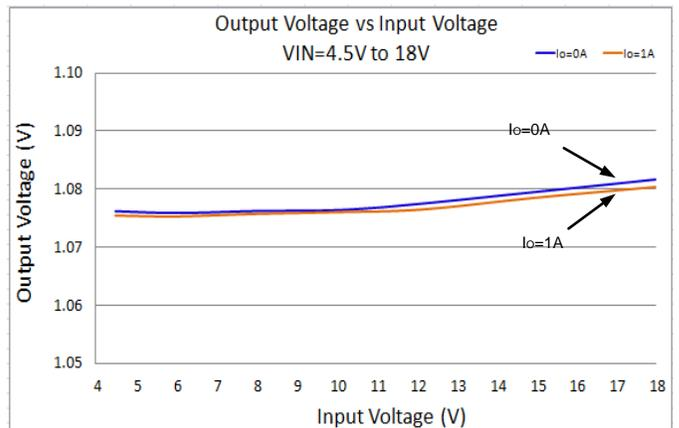
**Typical Performance Characteristics** (continued) (@ $T_A = +25^\circ\text{C}$ ,  $V_{IN} = 12\text{V}$ ,  $V_{OUT} = 1.05\text{V}$ , unless otherwise specified.)
