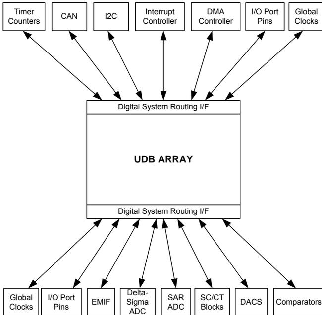
Interrupt and DMA routing is very flexible in the CY8C56LP programmable architecture. In addition to the numerous fixed function peripherals that can generate interrupt requests, any data signal in the UDB array routing can also be used to generate a request. A single peripheral may generate multiple independent interrupt requests simplifying system and firmware design. Figure 7-10 shows the structure of the IDMUX (Interrupt/DMA Multiplexer).
