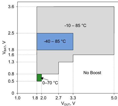
Figure 11-9. I<sub>OUT</sub> range over V<sub>BAT</sub> and V<sub>OUT</sub>
