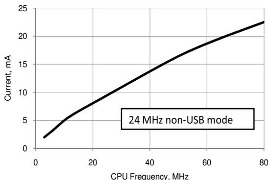
**Figure 11-2.  $I_{DD}$  vs Frequency at 25 °C**
