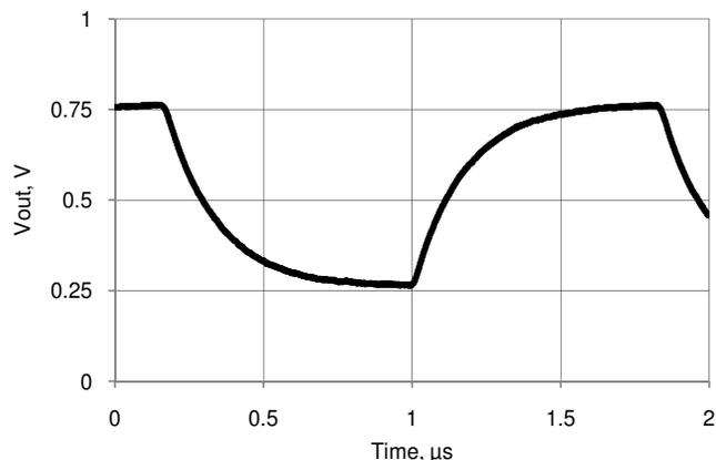
**Figure 11-65. VDAC Glitch Response, Codes 0x7F - 0x80, 1 V Mode, Fast Mode, V<sub>DDA</sub> = 5 V**
