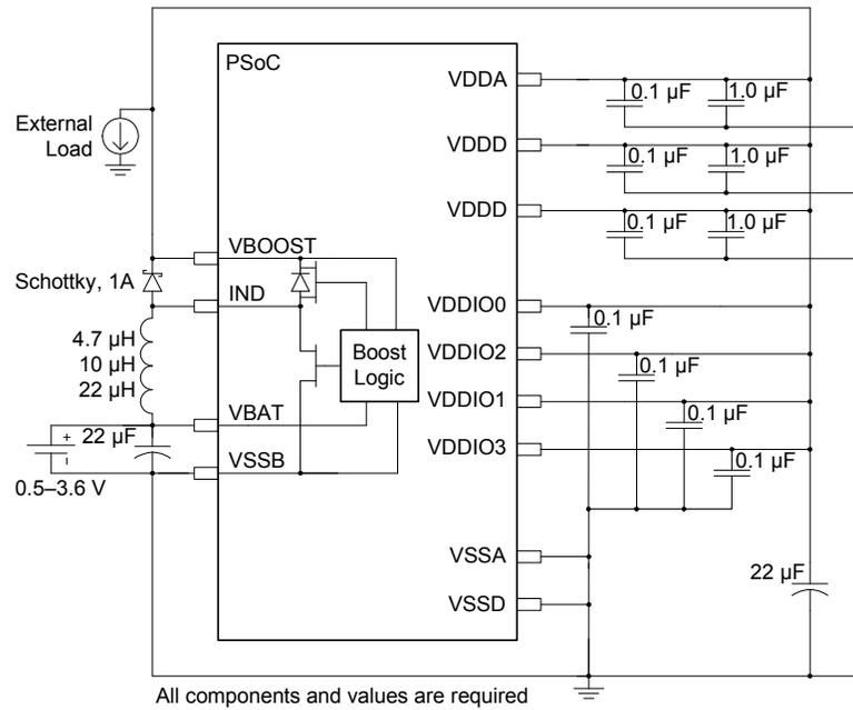
The boost converter may also generate a supply that is not used directly by the PSoC device. An example of this use case is boosting a 1.8 V supply to 4.0 V to drive a white LED. If the boost converter is not supplying the PSoC devices  $V_{DDA}$ ,  $V_{DDD}$ , and  $V_{DDIO}$  it must comply with the same design rules as supplying
