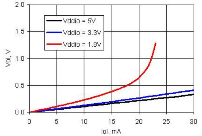
**Figure 11-19. SIO Output High Voltage and Current, Regulated Mode**
