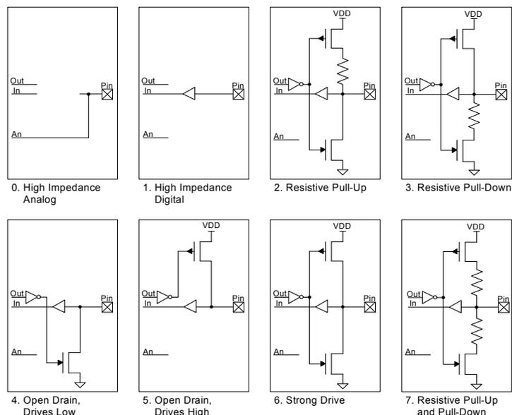
The 'Out' connection is driven from either the Digital System (when the Digital Output terminal is connected) or the Data Register (when HW connection is disabled).
