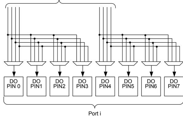
There are four more DSI connections to a given I/O port to implement dynamic output enable control of pins. This connectivity gives a range of options, from fully ganged 8-bits controlled by one signal, to up to four individually controlled pins. The output enable signal is useful for creating tri-state bidirectional pins and buses.
