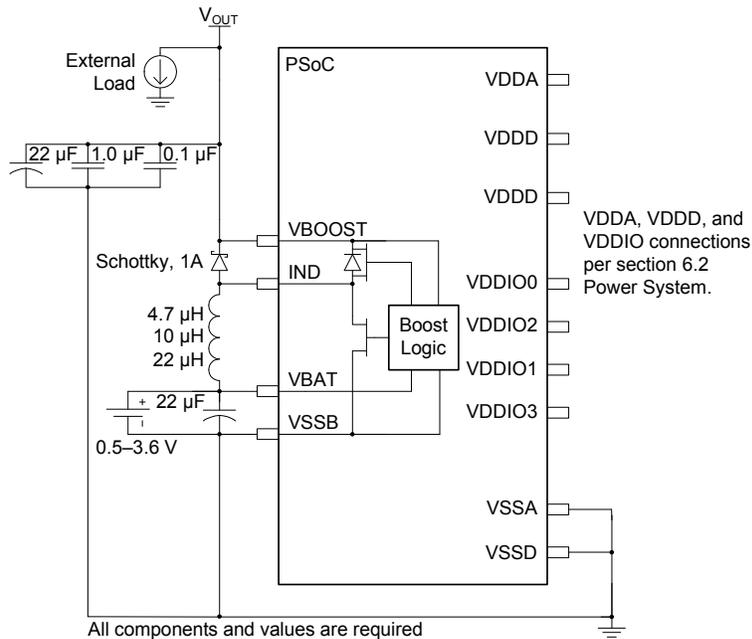
The switching frequency is set to 400 kHz using an oscillator integrated into the boost converter. The boost converter can be operated in two different modes: active and standby. Active
