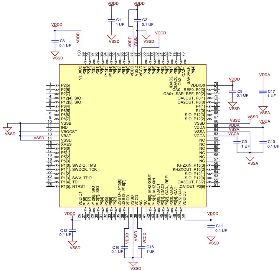
**Note** The two VCCD pins must be connected together with as short a trace as possible. A trace under the device is recommended, as shown in Figure 2-6.
