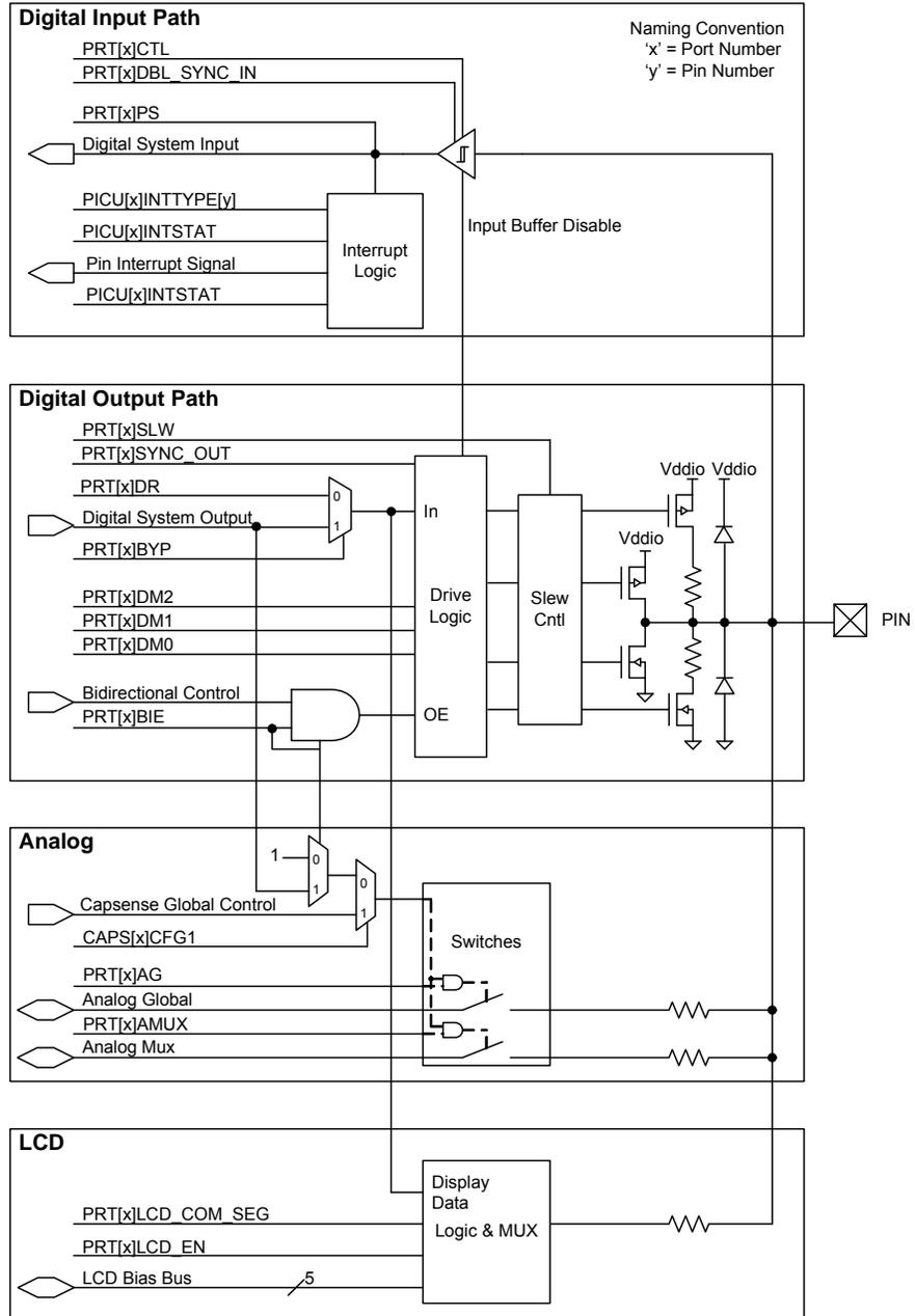
Figure 6-10. SIO Input/Output Block Diagram
