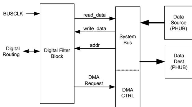
The typical use model is for data to be supplied to the DFB over the system bus from another on-chip system data source such as an ADC. The data typically passes through main memory or is directly transferred from another chip resource through DMA.
