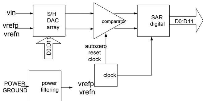
The input is connected to the analog globals and muxes. The frequency of the clock is 18 times the sample rate; the clock rate ranges from 1 to 18 MHz.
