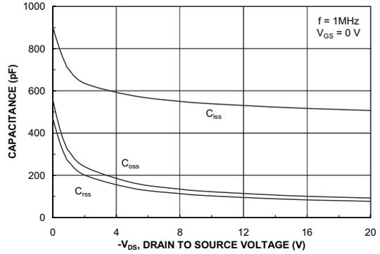
Figure 8. Capacitance Characteristics.
