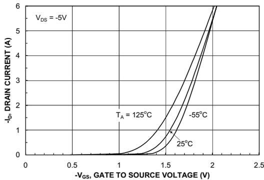
Figure 5. Transfer Characteristics.
