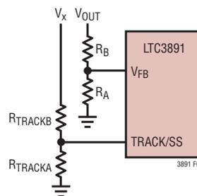
Figure 7. Using the TRACK/SS Pin for Tracking
