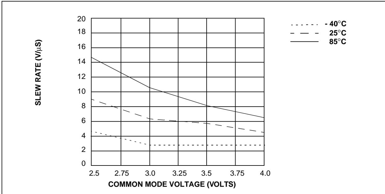
**FIGURE 3: VOLTAGE COMPARATOR INPUT, MAXIMUM SLEW RATE AT  $V_{DD} = 4.0V$**
