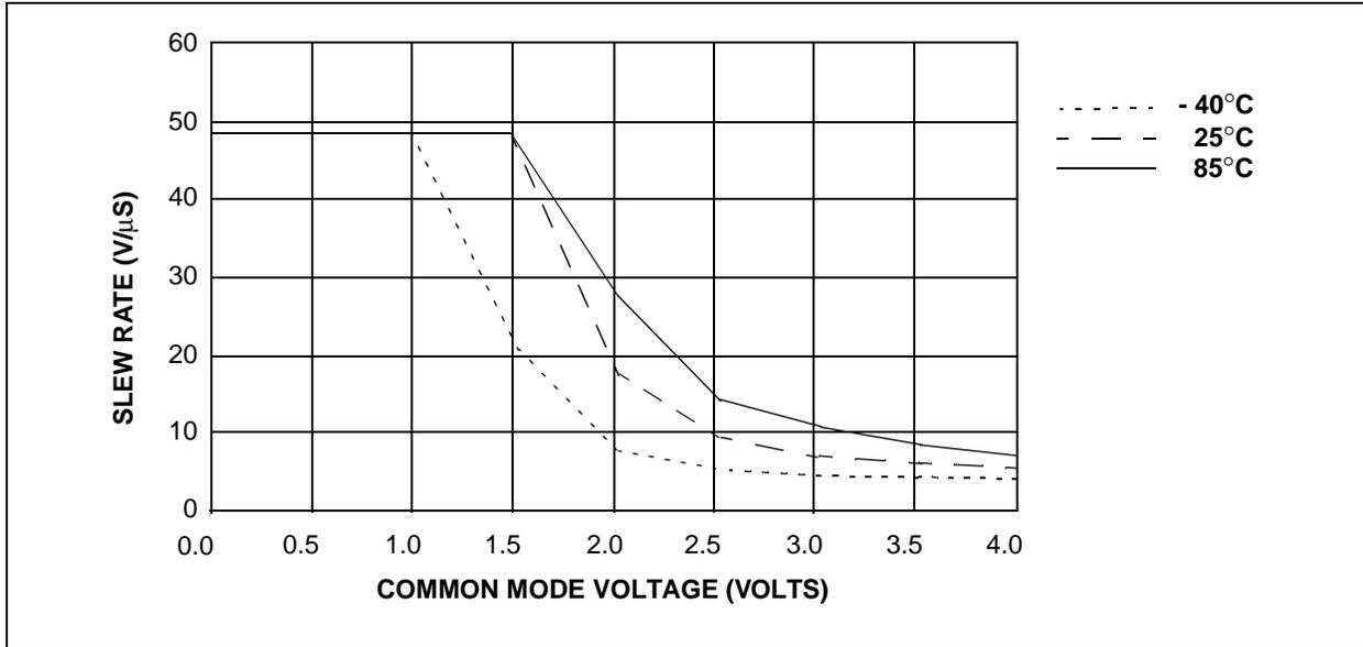
FIGURE 2: VOLTAGE COMPARATOR INPUT, MAXIMUM SLEW RATE AT  $V_{DD} = 5.5V$
