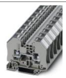
Feed-through terminal block with bolt connection technology and transparent safety contact hood, cross section: 0.1 - 6 mm², AWG: 26 - 10, width 16.3 mm, color: gray
