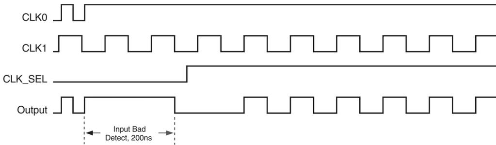
**Figure 1D. CLK\_SEL with Bad Input Timing Diagram**
