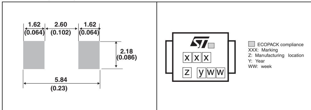
1. Product marking may be rotated by 90° for assembly plant differentiation. In no case should this product marking be used to orient the component for its placement on a PCB. Only pin 1 mark is to be used for this purpose.
