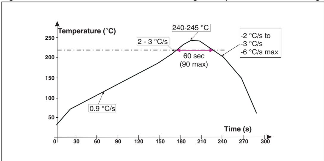
Note: Minimize air convection currents in the reflow oven to avoid component movement.
