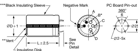
**VS, VE & VN Snap-in Pin Dimensions**
