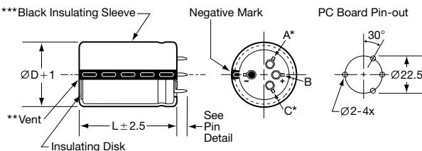
**VNT Snap-in Ø45 and Ø50 standard**
