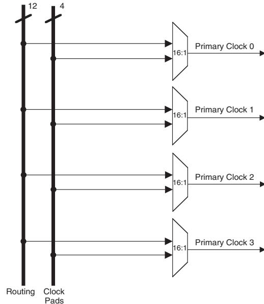
**Figure 2-8. Primary Clocks for LA-MachXO1200 and LA-MachXO2280 Devices**
