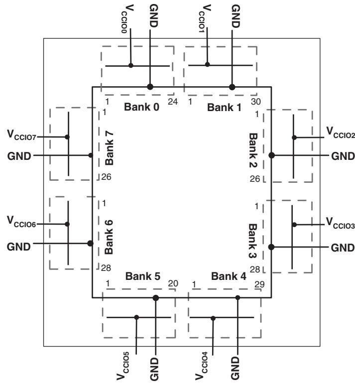
**Figure 2-20. LA-MachXO640 Banks**
