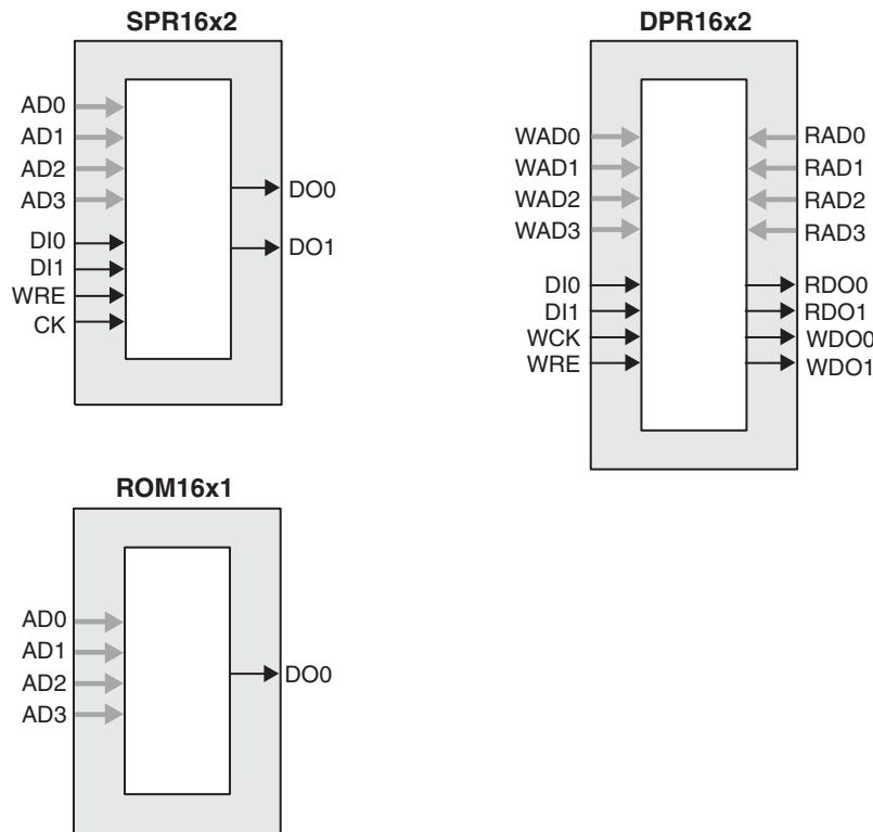
**ROM Mode:** The ROM mode uses the same principal as the RAM modes, but without the Write port. Pre-loading is accomplished through the programming interface during configuration.
