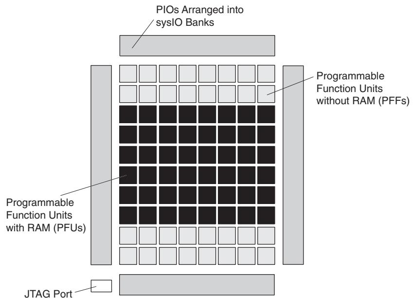
**Figure 2-3. Top View of the LA-MachXO256 Device**
