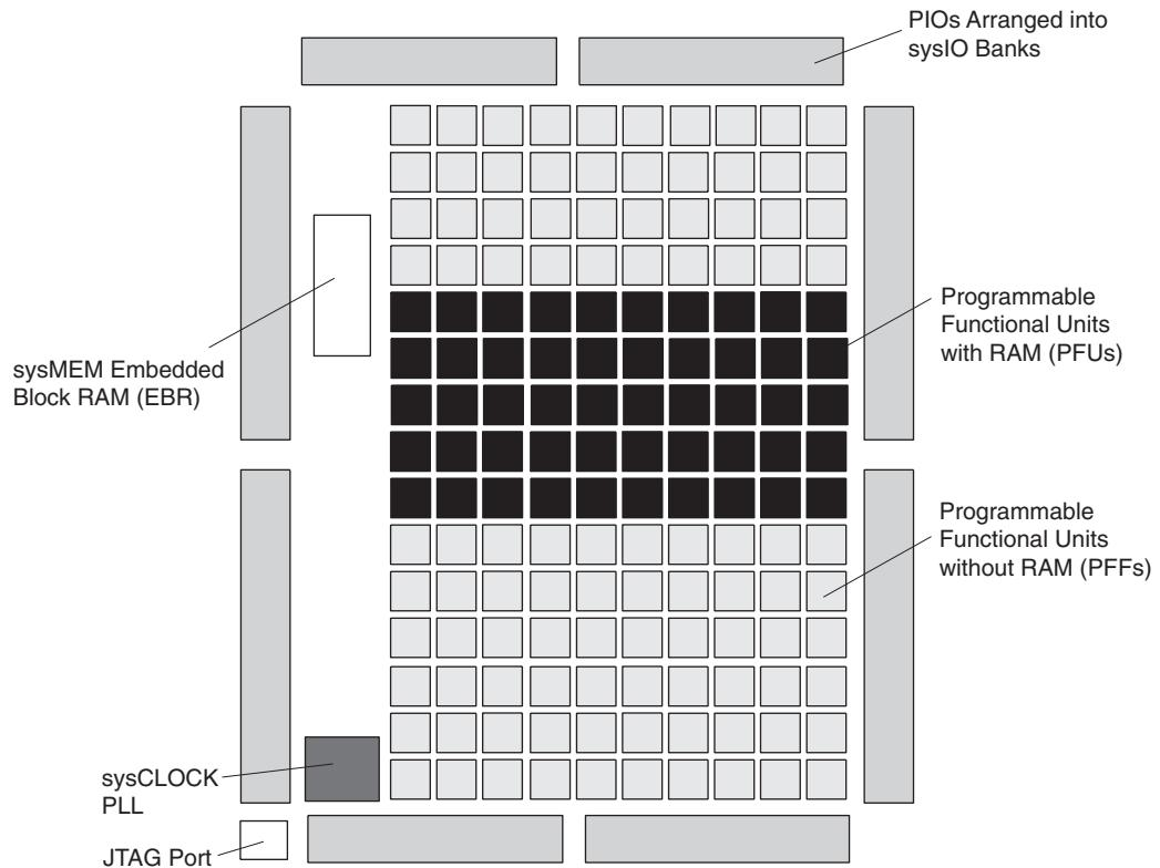
1. Top view of the LA-MachXO2280 device is similar but with higher LUT count, two PLLs, and three EBR blocks.
