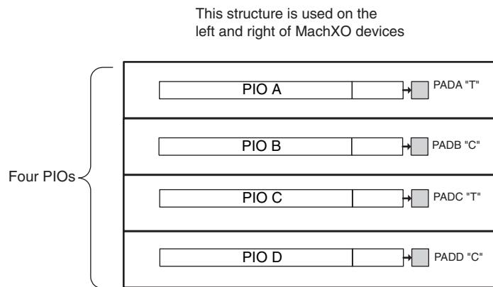
**Figure 2-16. Group of Six Programmable I/O Cells**
