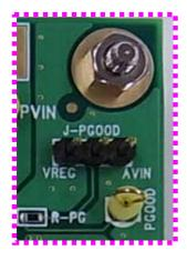
Table 4. J-PGOOD (Control the Voltage PGOOD pin pulled up to)
