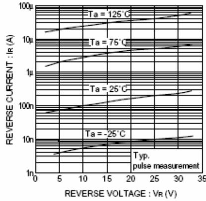
Fig. 2 Reverse characteristics
