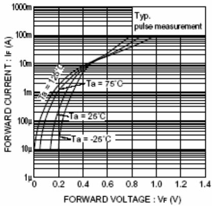
Fig. 1 Forward characteristics
