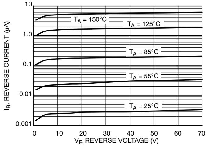
Figure 3. Leakage Current
