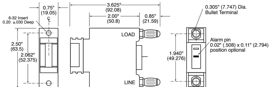
Dimensions for reference only. For additional options and dimensions, contact the factory.
