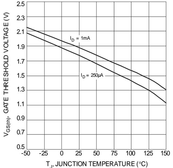
Figure 8 Gate Threshold Variation vs. Ambient Temperature
