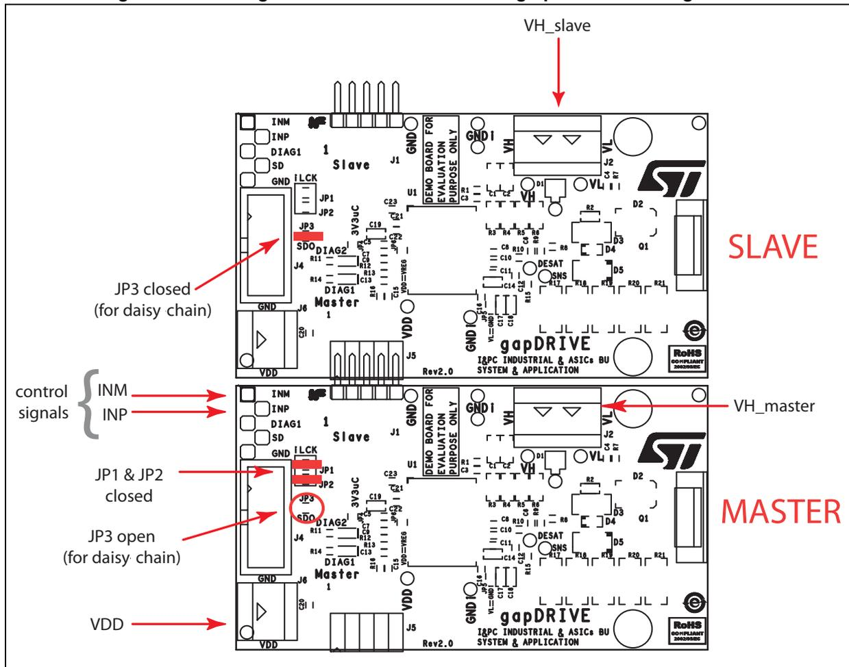
Figure 8. Half bridge with independent input signal configurations
