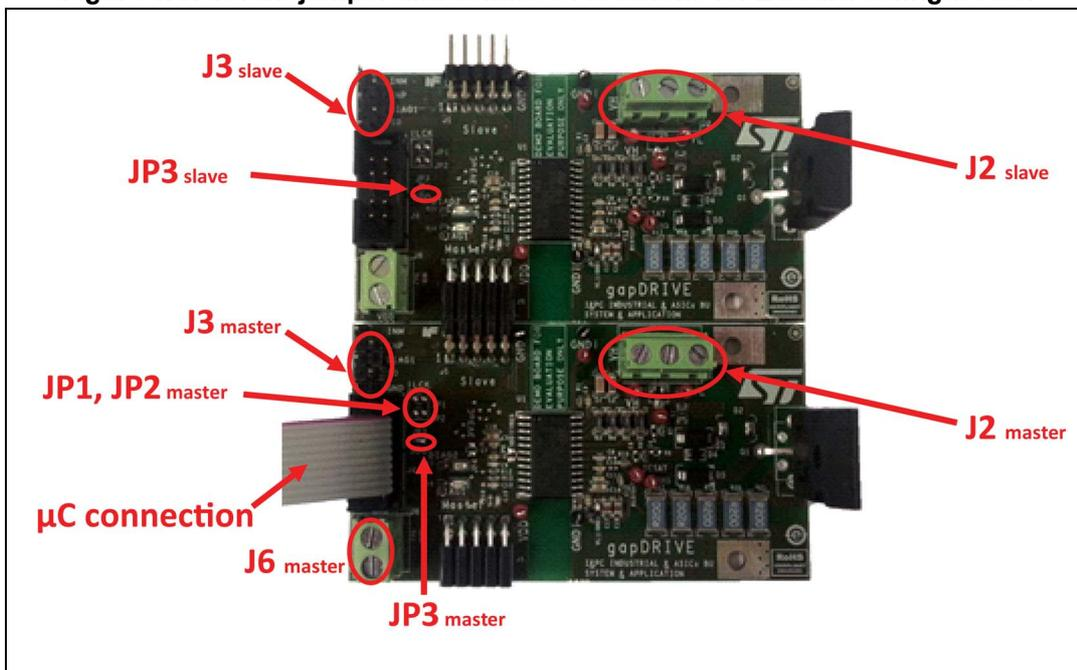
Connecting two EVALSTGAP1S boards allows implementing independent, half bridge, or interleaved configuration of power switches  $Q1_m$  and  $Q1_s$ .
