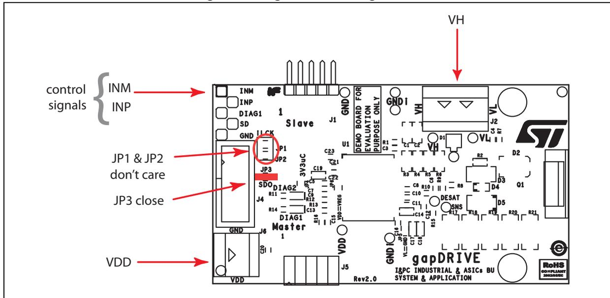
Figure 7. Half bridge with hardware shoot-through protection configuration
