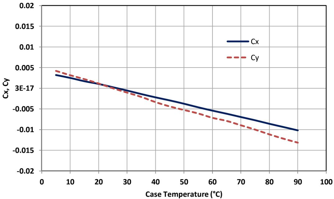
Figure 6: Typical dominant wavelength shift vs. Case temperature.
