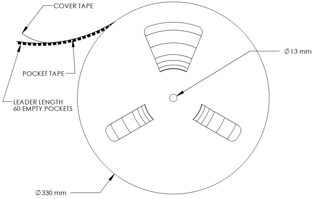
Figure 12: Emitter Reel specifications (mm).
