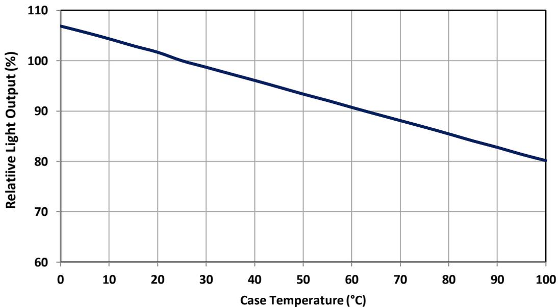
Figure 8: Typical relative light output vs. case temperature.
