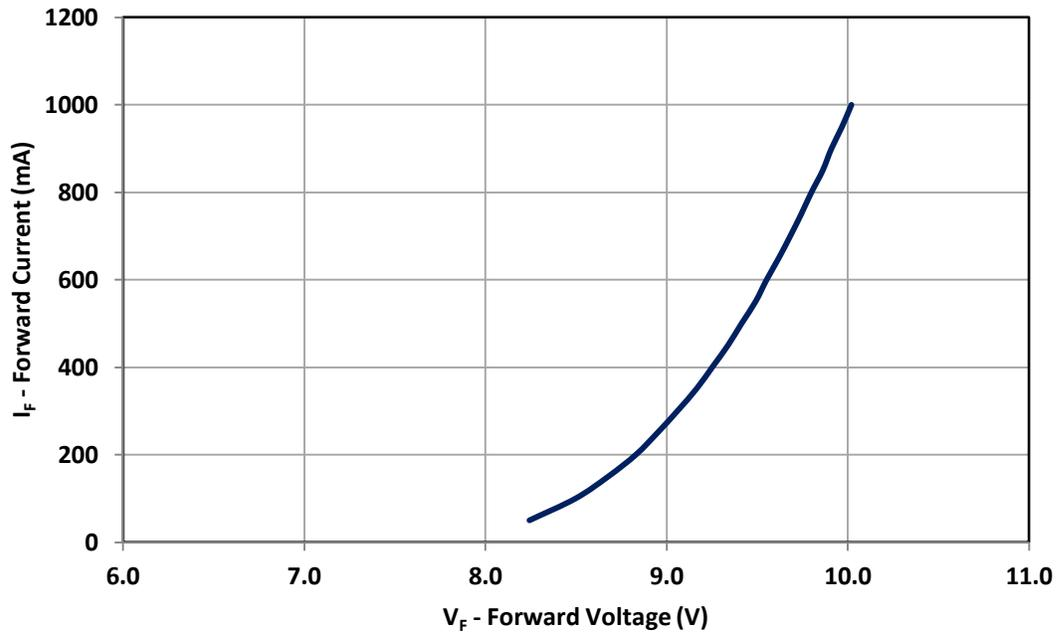
Figure 9: Typical forward current vs. forward voltage<sup>1</sup> @  $T_c = 25^\circ\text{C}$ .
