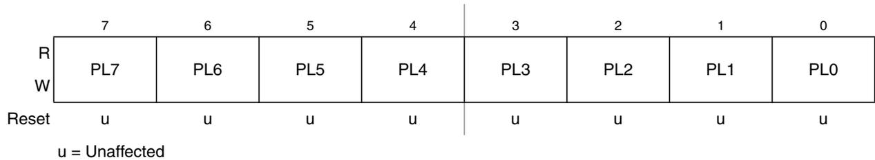
Figure 8-9. Carrier Generator Data Register Low 1 (CMTCGL1)
