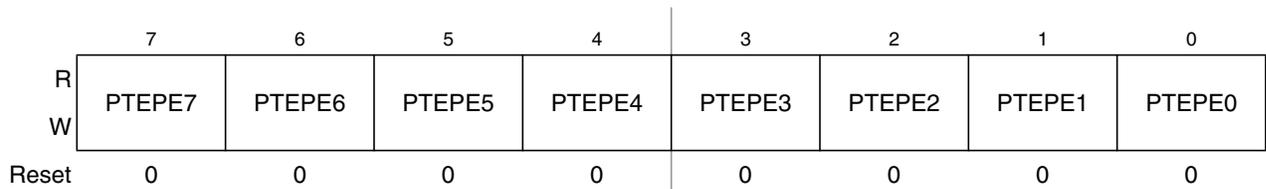
Figure 6-19. Pullup Enable for Port E (PTEPE)
