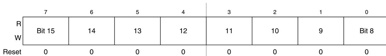
Figure 10-11. Timer Channel Value Register High (TPM1CnVH)
