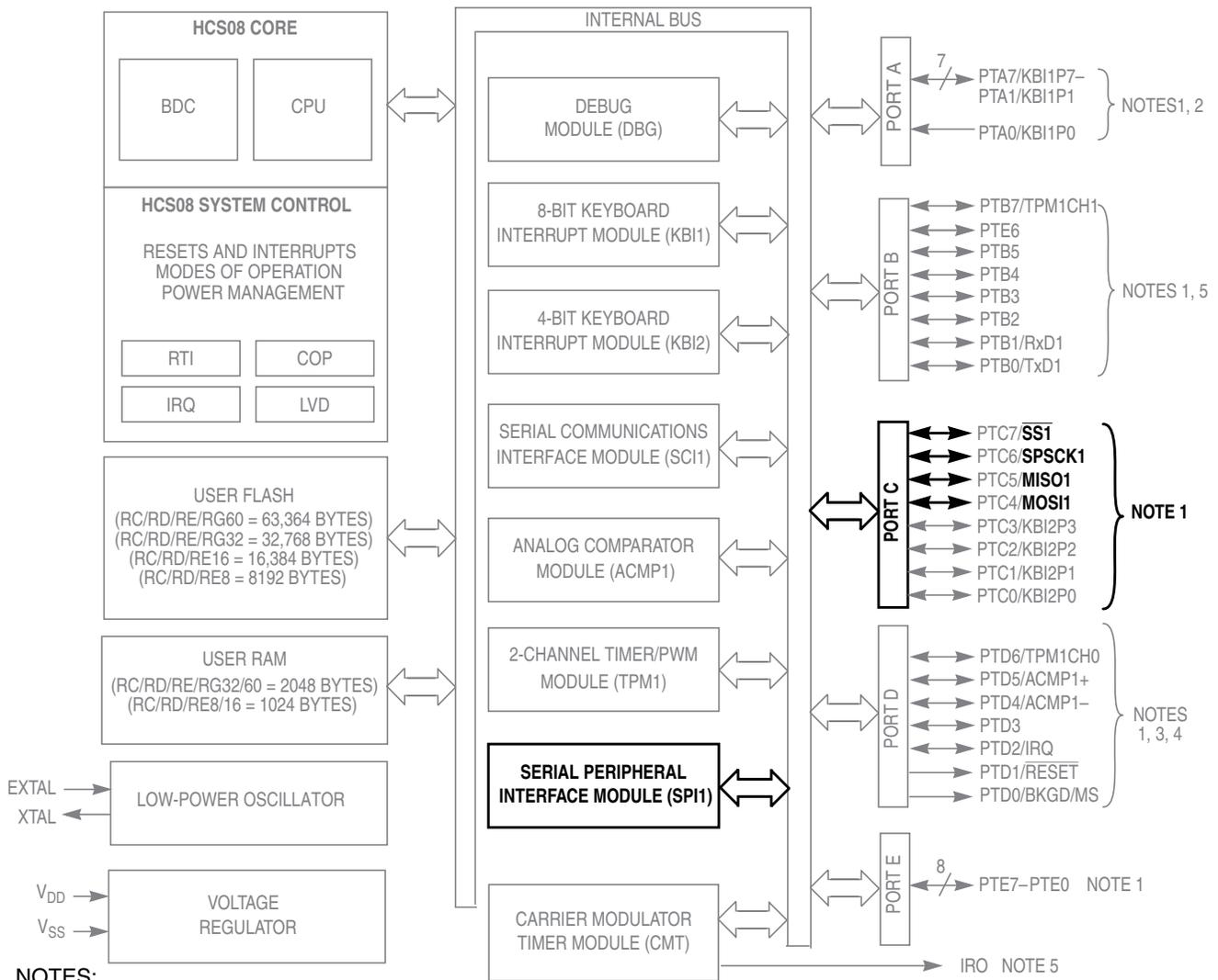
**Figure 13-1. MC9S08RC/RD/RE/RG Block Diagram Highlighting SPI Block and Pins**
