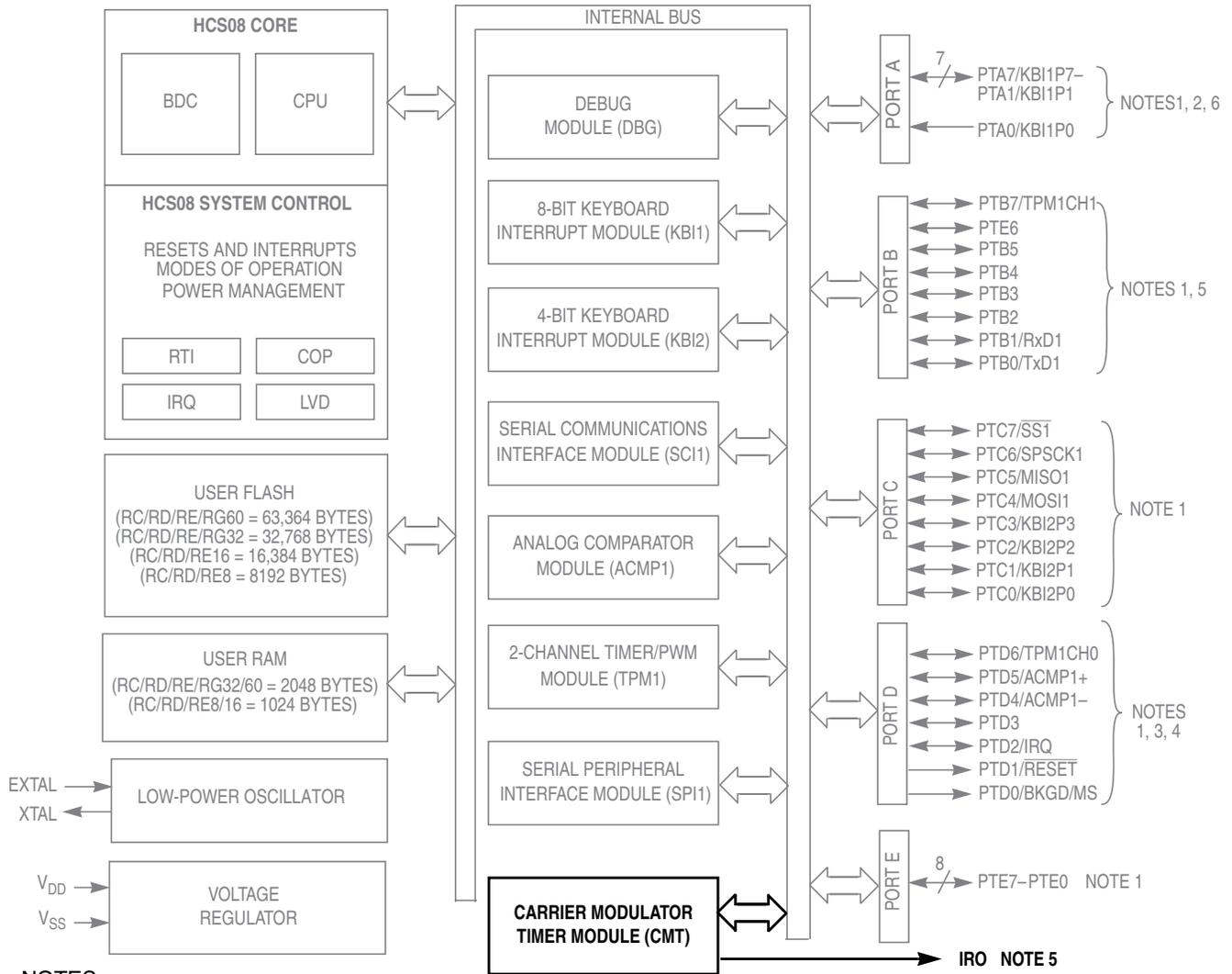
Figure 8-1. MC9S08RC/RD/RE/RG Block Diagram
