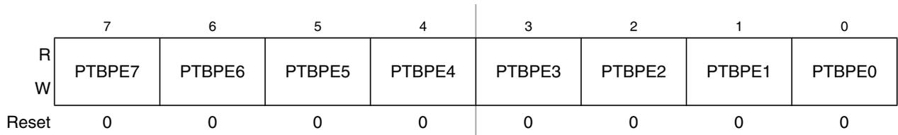
Figure 6-10. Pullup Enable for Port B (PTBPE)
