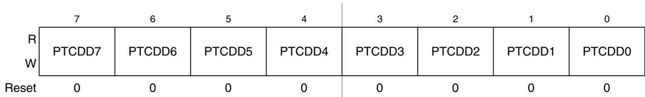
Figure 6-14. Data Direction for Port C (PTCDD)
