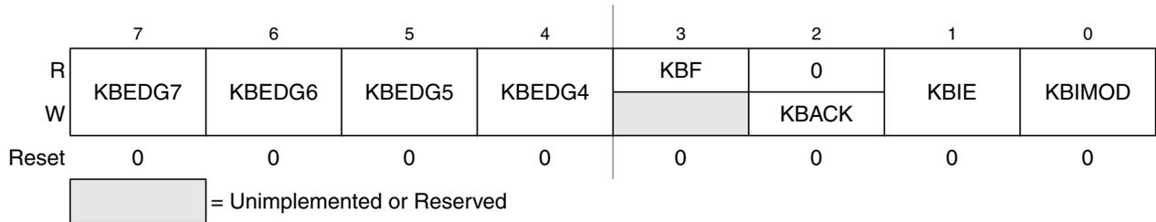
Figure 9-3. KBI x Status and Control Register (KBIXSC)
