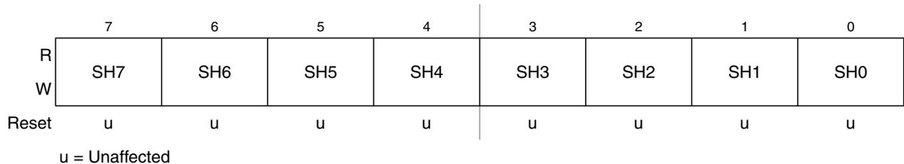
Figure 8-10. Carrier Generator Data Register High 2 (CMTCGH2)
