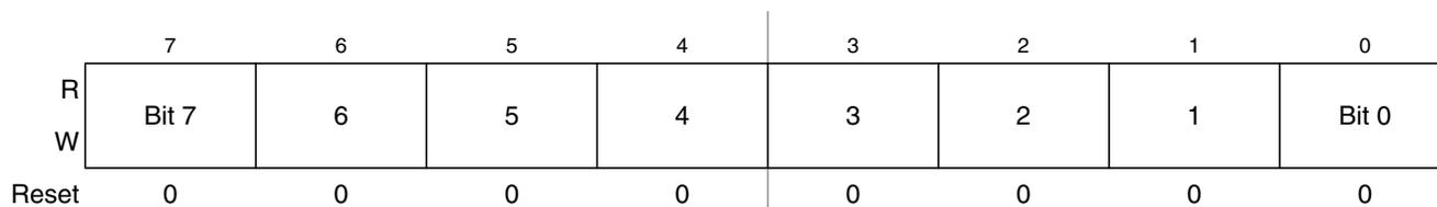
Figure 10-12. Timer Channel Value Register Low (TPM1CnVL)
