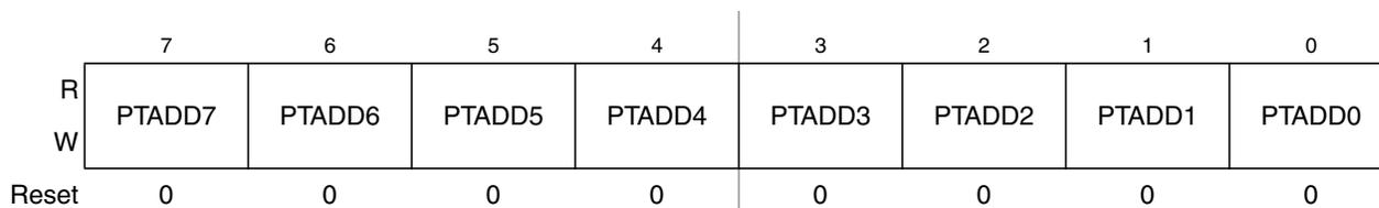
Figure 6-8. Data Direction for Port A (PTADD)
