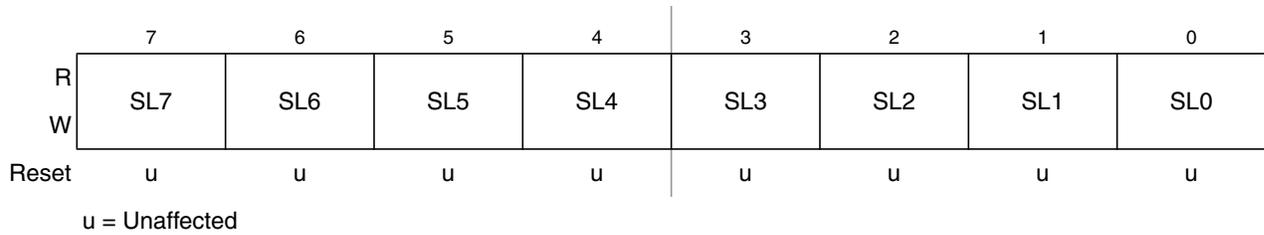
**Figure 8-11. Carrier Generator Data Register Low 2 (CMTCGL2)**
