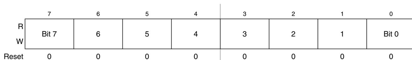
Figure 10-9. Timer Counter Modulo Register Low (TPM1MODL)
