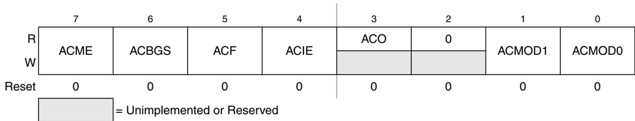
Figure 14-3. ACMP Status and Control Register (ACMP1SC)
