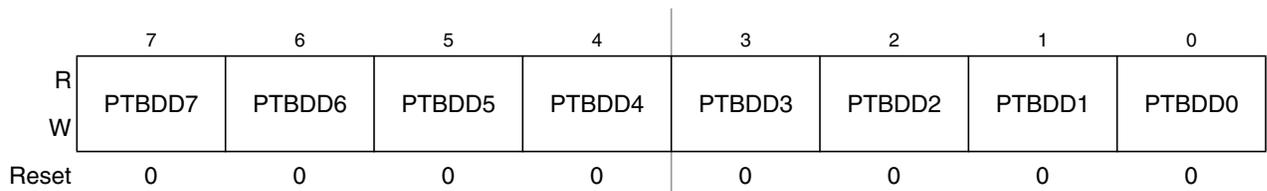
Figure 6-11. Data Direction for Port B (PTBDD)
