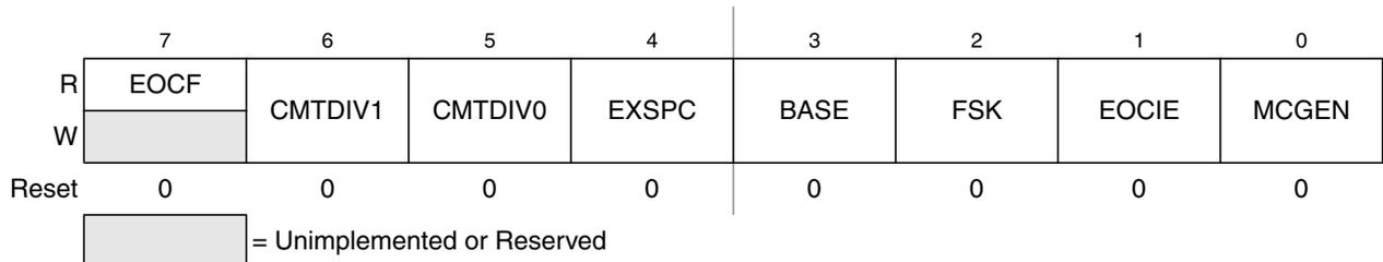
Figure 8-13. CMT Modulator Status and Control Register (CMTMSC)
