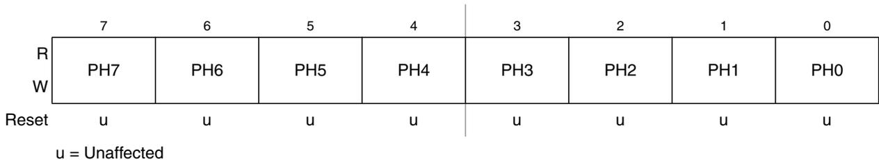
**Figure 8-8. Carrier Generator Data Register High 1(CMTCGH1)**
