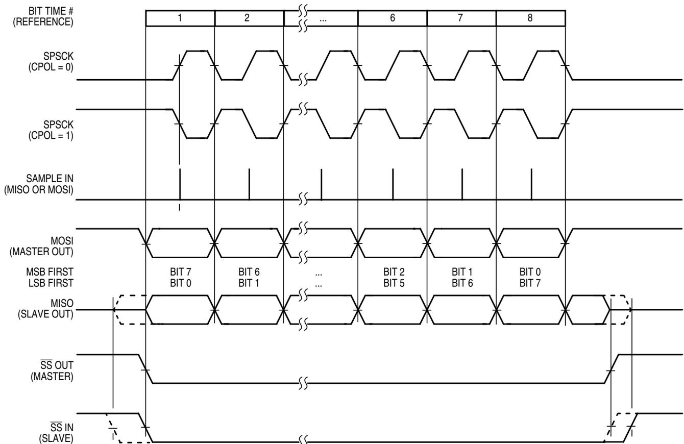
Figure 13-6. SPI Clock Formats ( $CPHA = 0$ )
