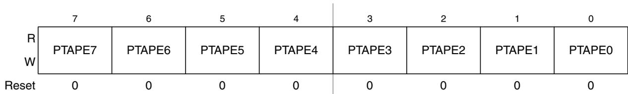
Figure 6-7. Pullup Enable for Port A (PTAPE)
