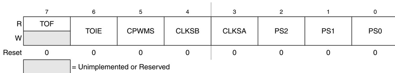
**Figure 10-5. Timer Status and Control Register (TPM1SC)**
