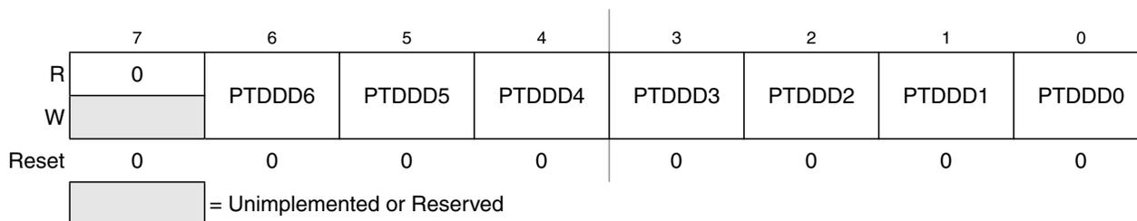
Figure 6-17. Data Direction for Port D (PTDDD)
