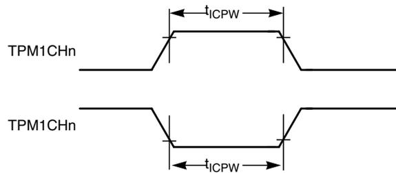
**Figure A-10. Timer Input Capture Pulse**
