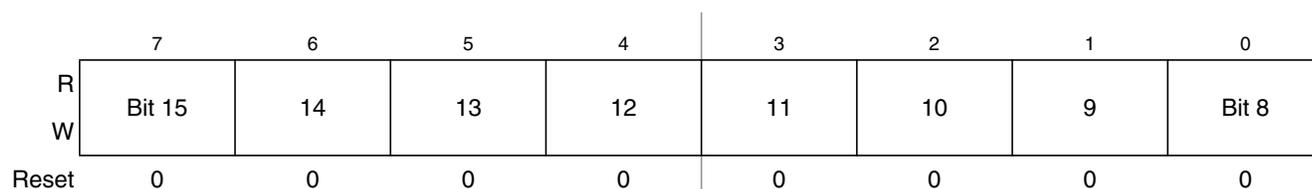
Figure 10-8. Timer Counter Modulo Register High (TPM1MODH)
