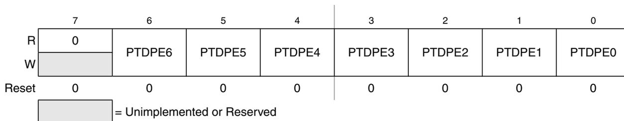
Figure 6-16. Pullup Enable for Port D (PTDPE)
