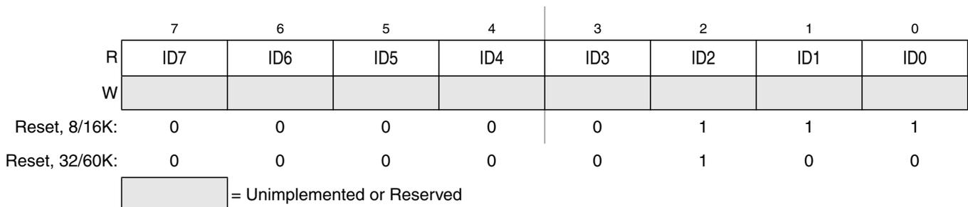
**Figure 5-7. System Device Identification Register — Low (SDIDL)**
