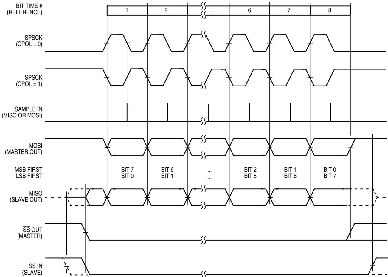
Figure 13-5. SPI Clock Formats (CPHA = 1)
