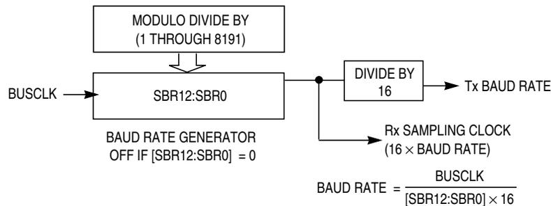
Figure 12-11. SCI Baud Rate Generation
