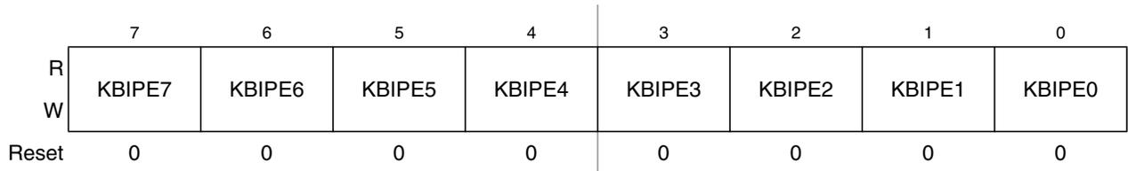
Figure 9-4. KBI x Pin Enable Register (KBIXPE)
