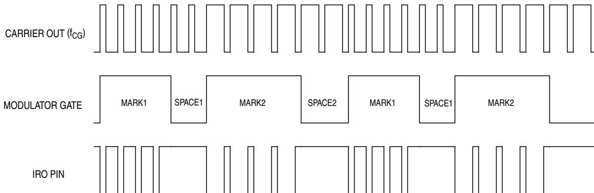
Figure 8-6. Example CMT Output in FSK Mode
