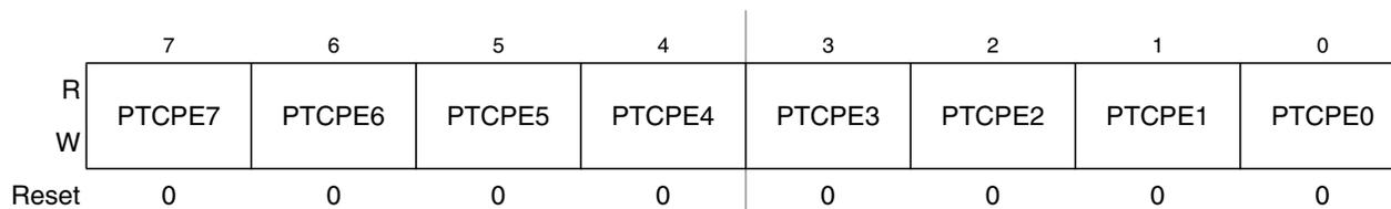
Figure 6-13. Pullup Enable for Port C (PTCPE)
