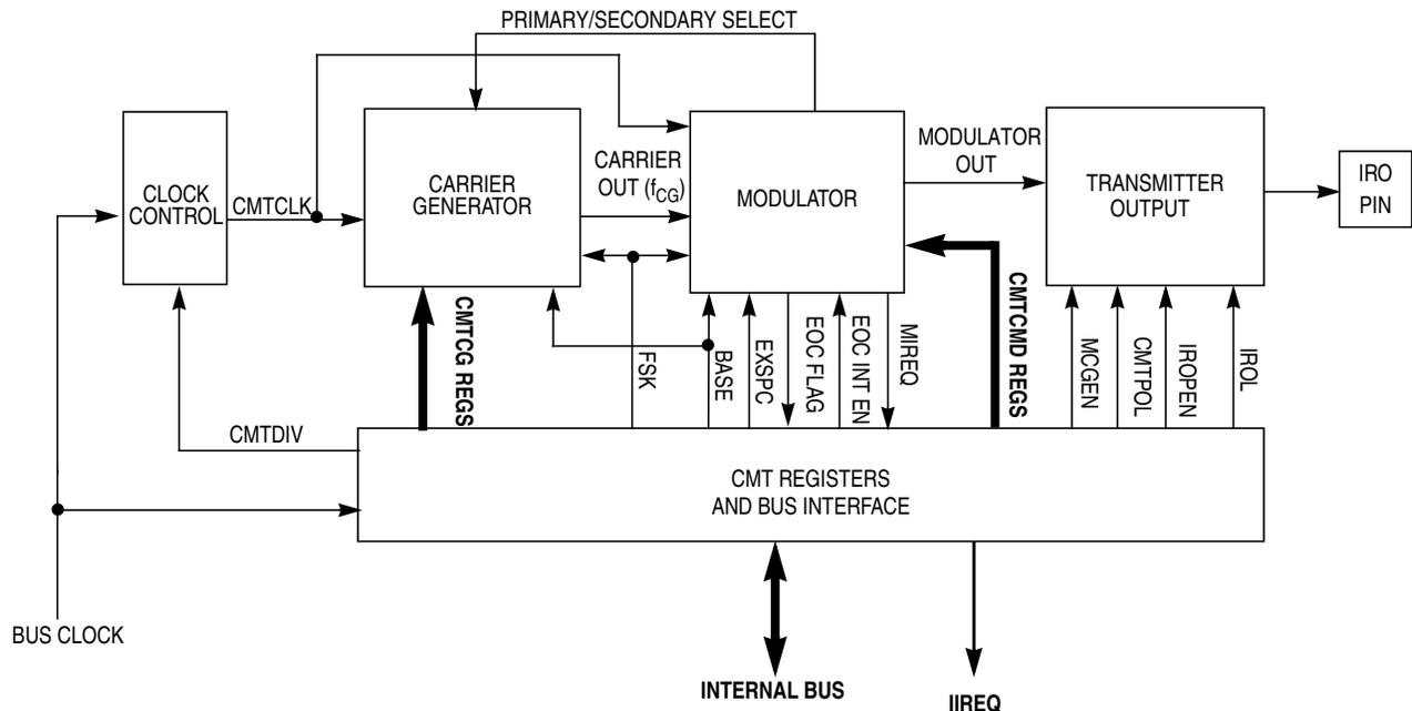
Figure 8-2. Carrier Modulator Transmitter Module Block Diagram
