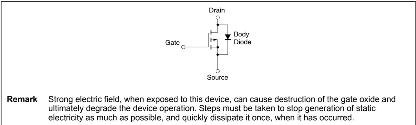
**Remark** Strong electric field, when exposed to this device, can cause destruction of the gate oxide and ultimately degrade the device operation. Steps must be taken to stop generation of static electricity as much as possible, and quickly dissipate it once, when it has occurred.
