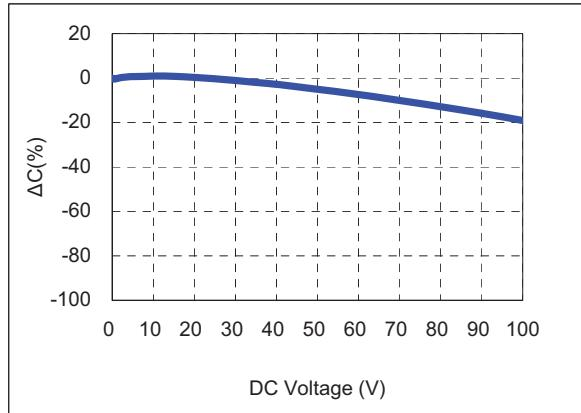
4) Bias TCC characteristics (Agilent 4284A, 1kHz, 1Vrms, 50Vdc)
