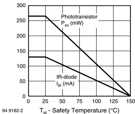
Fig. 1 - Derating Diagram
