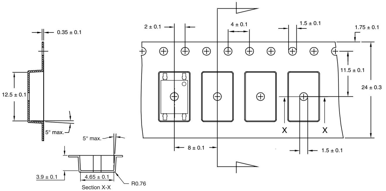
Fig. 8 - Tape and Reel Packing for Option 8
