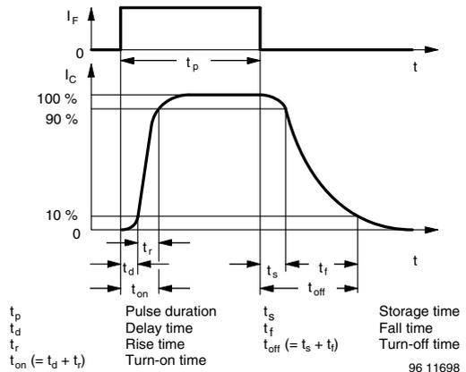
Fig. 5 - Switching Times
