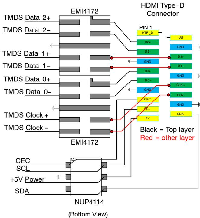
Figure 16. EMI4172 HDMI Type – D Connector Application Diagram
