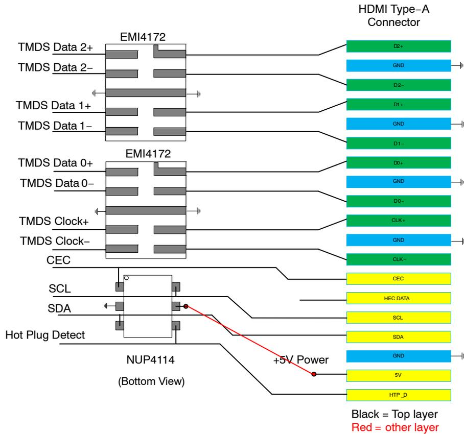
Figure 15. EMI4172 HDMI Type – A Connector Application Diagram
