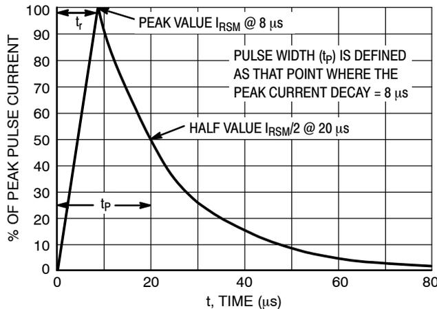
Figure 12. 8 x 20  $\mu s$  Pulse Waveform
