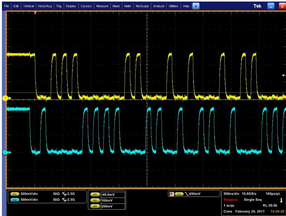
Figure 5. EMI4172 MIPI D-PHY LP Mode Measured Results
