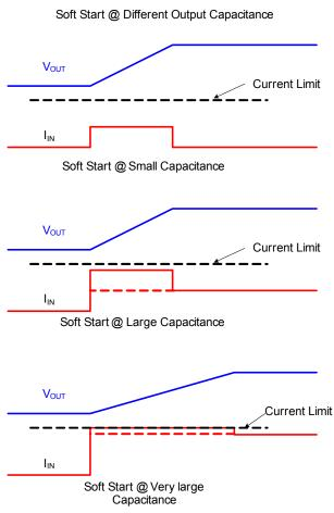
Figure 3: Soft Start Periods at different output capacitance
