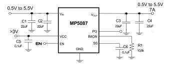
Figure 4: Typical Application Schematic
