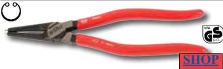
**326 Straight Internal Retaining Ring Pliers** DIN ISO 5256 Shape C, straight tips. Die forged cylindrical precision formed. Chrome-vanadium special tool steel. For inserting & removing internal retaining rings.
