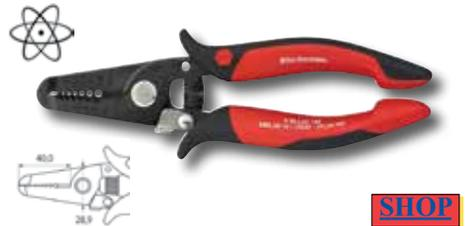
**56871 Stripping Pliers** Wide long head with ridged gripping surface, shears blade and firm wire stripping stations. With opening spring and locking mechanism. Wire stripping stations 0.81 / 1.0 / 1.3 / 1.6 / 2.0 / 2.59mm, AWG 20 / 18 / 16 / 14 / 12 / 10.
