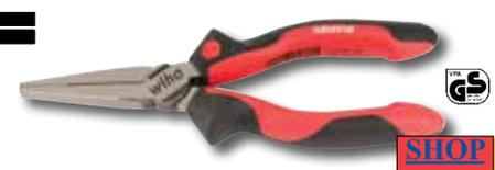
**30919 Industrial Long Flat Nose Pliers** DIN ISO 5745 Extra long head. Gripping surfaces serrated and induction hardened. C70 Special tool steel. Two component SoftGrip handle. Gripping and right-angled bending of wires and sheet metal parts.
