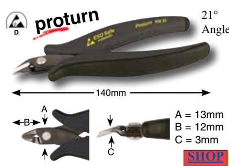
**45822 Protturn ESD Safe 21° Precision Cutters/Flush Cut** ESD standard IEC 61340-5-1. C70 special tool steel. Glare free, black finish. ESD Safe handle with non-slip grips.
