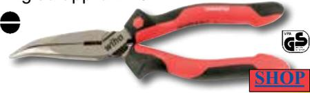
**309 Industrial Bent Nose Pliers With Cutters** DIN ISO 5745 Long nose pliers angled approx. 40°. Extra long cutting edge for flat & round wires. Gripping surfaces serrated in parts. Cutting edges additionally induction hardened to approx. 64HRC. C70 Special tool steel. Two component SoftGrip handle.
