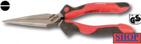
**309 Industrial Long Nose Pliers With Cutting Edge** DIN ISO 5745 Long nose pliers. Extra long cutters for flat and round wires. Gripping surfaces serrated in parts. Cutting edges additionally induction hardened to approx. 64HRC. C70 Special tool steel. Two component SoftGrip handle.
