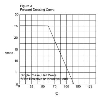
Average Forward Rectified Current - Amperes/ersus Case Temperature -  $^{\circ}$ C
