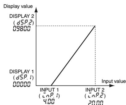
1. Set the K3MA-J input type to the 4 to 20 mA input range.
