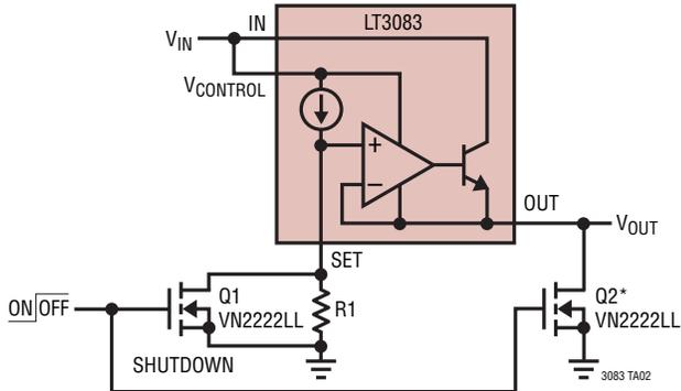
\*Q2 INSURES ZERO OUTPUT IN THE ABSENCE OF ANY OUTPUT LOAD.
