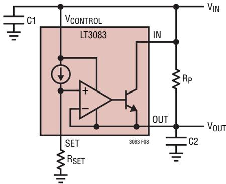
Figure 8. Reducing Power Dissipation Using a Parallel Resistor
