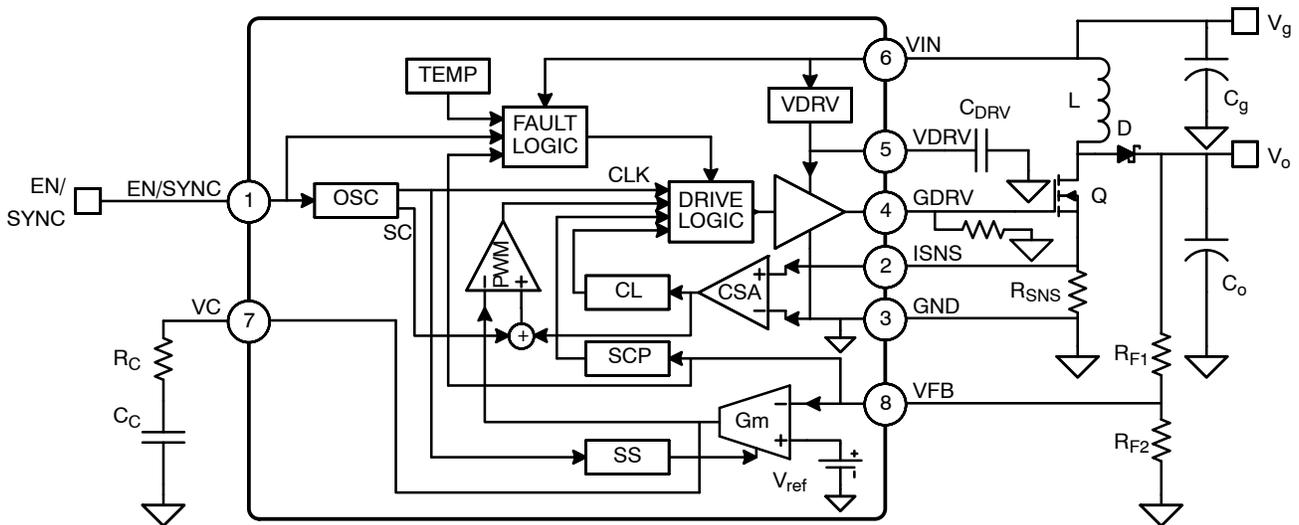
**Figure 1. Simplified Block Diagram and Application Schematic**
