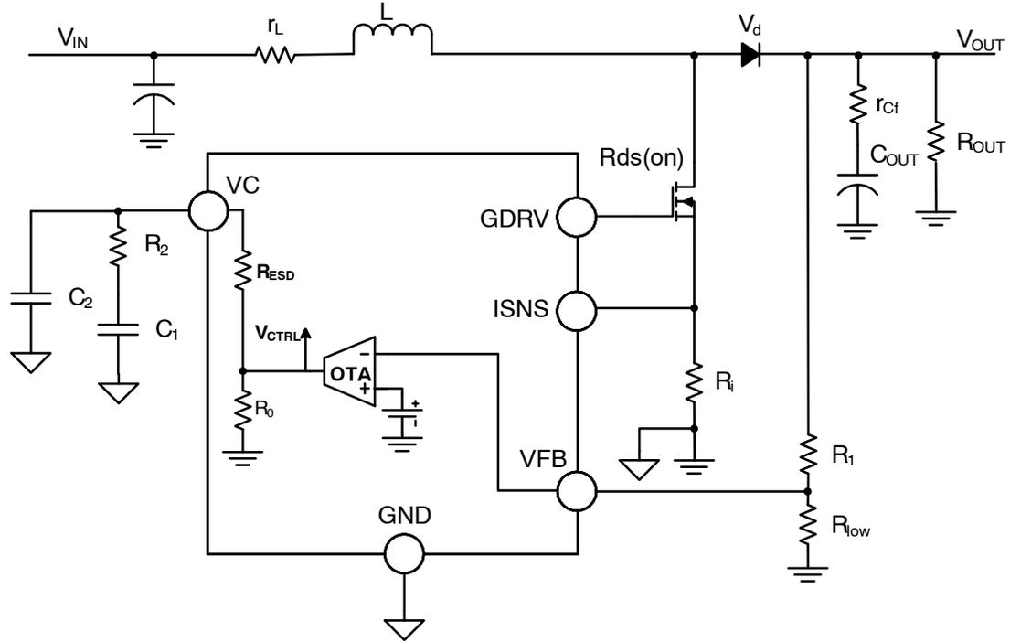
Figure 12. NCV887200 Boost Converter OTA and Compensation
