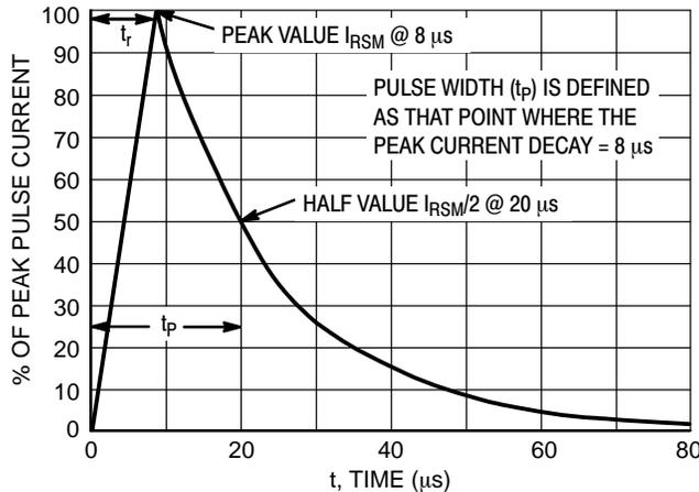
Figure 8. 8 X 20 μs Pulse Waveform
