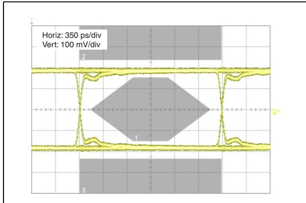
Figure 11. Eye diagram PCB + USBULC6-2M6
