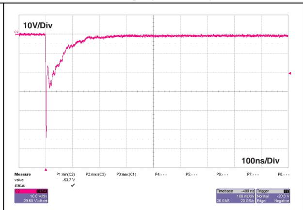
Figure 8. Remaining voltage on  $V_{BUS}$  after the USBULC6-2M6 during positive ESD surge (15 kV Air)
