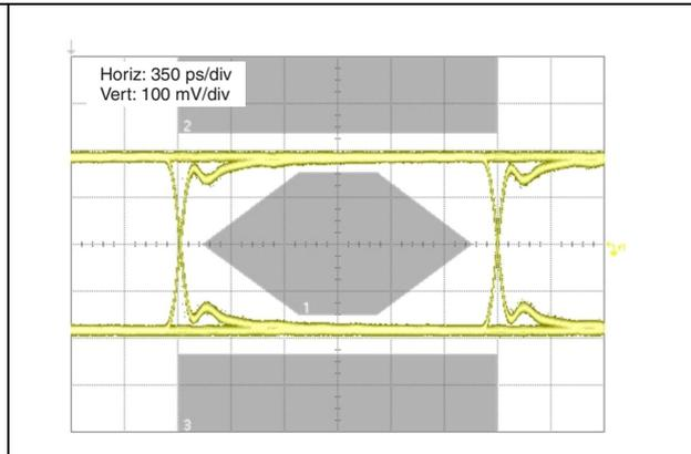
Figure 12. Eye diagram PCB + USBULC6-2M6, +5 V on  $V_{BUS}$  decoupling capacitor
