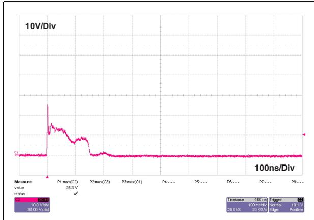
Figure 9. Remaining voltage on  $V_{BUS}$  after the USBULC6-2M6 during negative ESD surge (15 kV Air)
