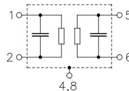
1) The recommended pin configuration usually offers best suppression of electrical crosstalk. The filter characteristics refer to this configuration.
