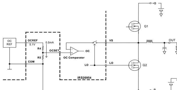
Since the sensed voltage of  $V_S$  is compared with the voltages fed to the OCSET pin, the required voltage of OCSET with respect to COM for a trip level  $I_{TRIP+}$  is:
