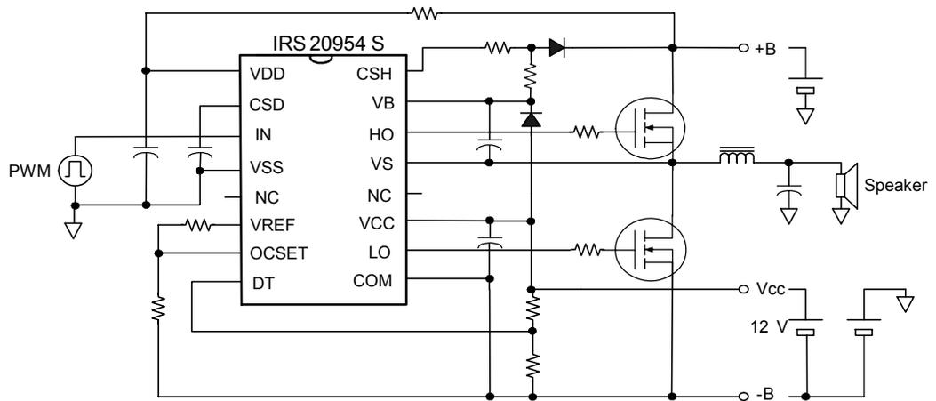
(Please refer to Lead Assignments for correct pin configuration. This diagram shows electrical connections only)
