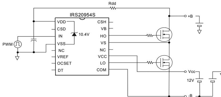
**Figure 18: Supplying V<sub>DD</sub>**
